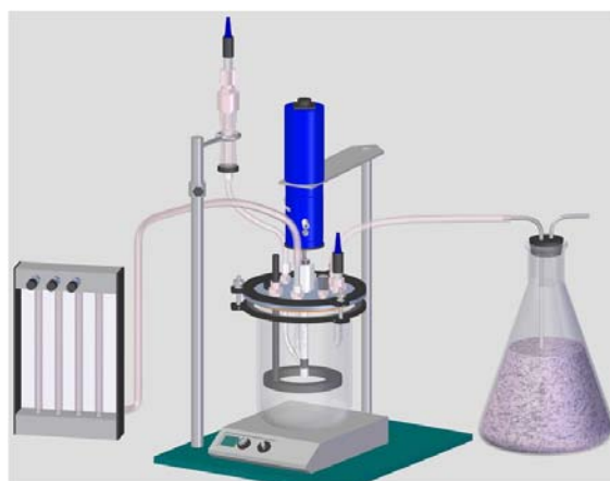
FIGURE 1 – Experimental Setup for Corrosion Tests
