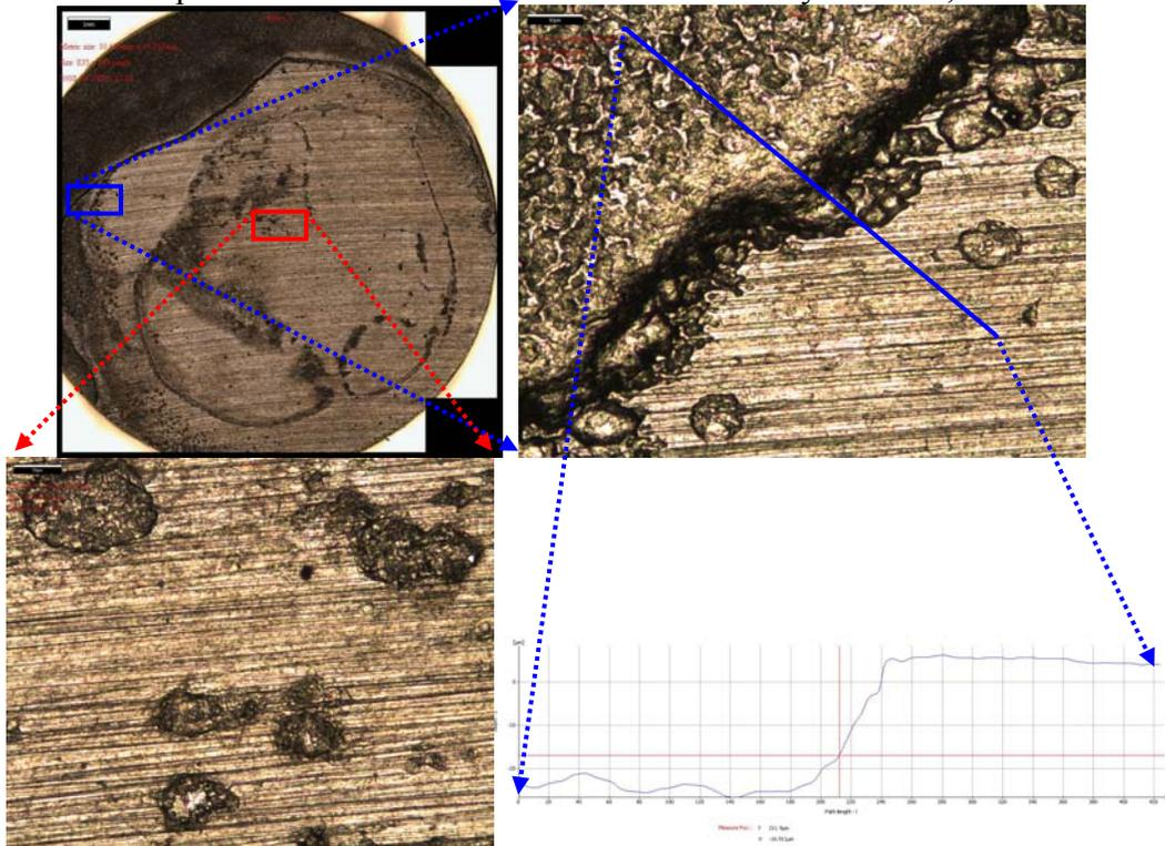
Figure 7. IFM data for coupon contacted with sulfur for 4 days at 25°C, without film, appearance of the surface and a line profile.
