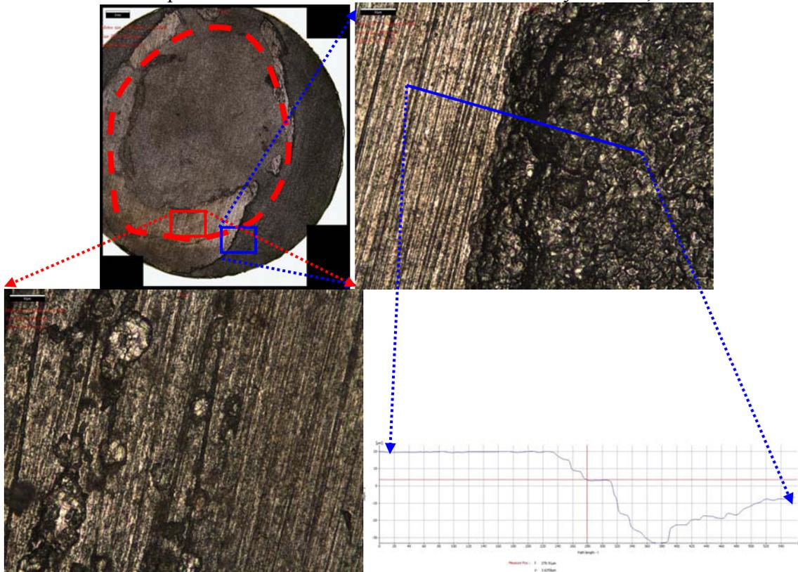
Figure 14. IFM data for coupon contacted with sulfur for 1 days at 80°C, without film, appearance of the surface and a line profile.
