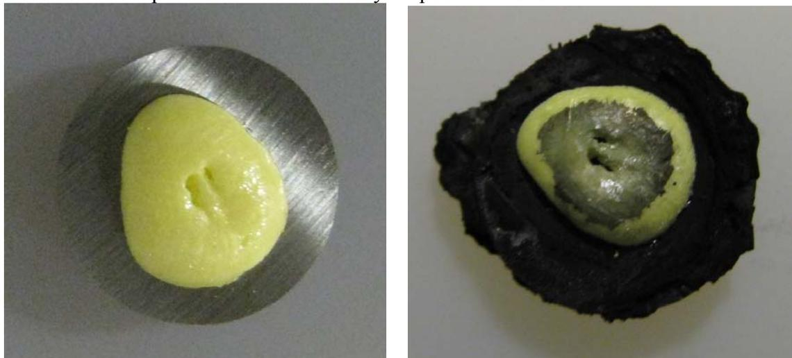
Figure 3. Corrosion coupon before and after 5 days exposure at 25°C.
