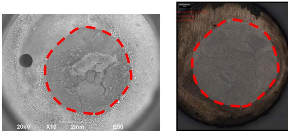
Figure 18. Corrosion coupon contacted with elemental sulfur for 4 days with and without film at 25°C, salt free condition
