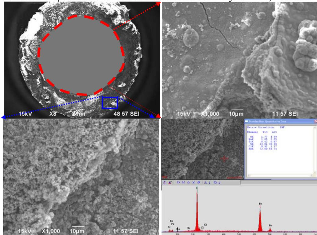
Figure 16. Corrosion coupon contacted with elemental sulfur for 5 days at 80°C, with film.
