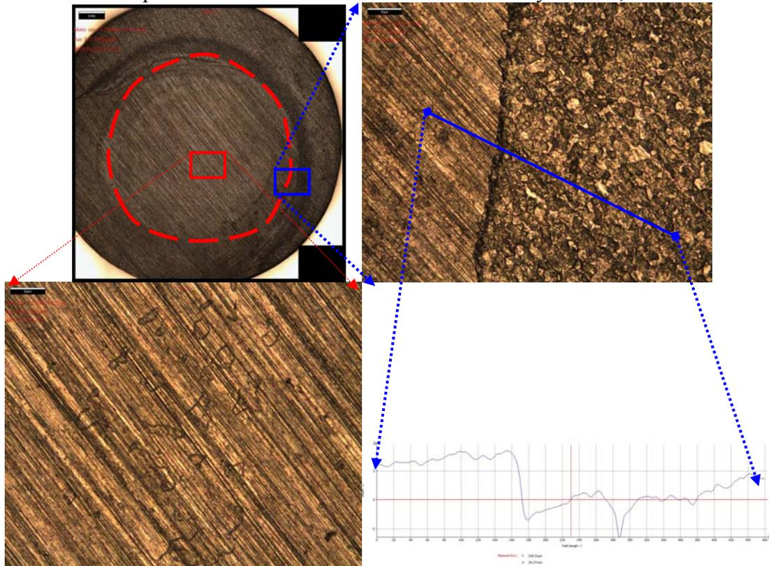
Figure 5. IFM data for corrosion coupon for 1 day at 25°C, without film, appearance of the surface and a line profile.
