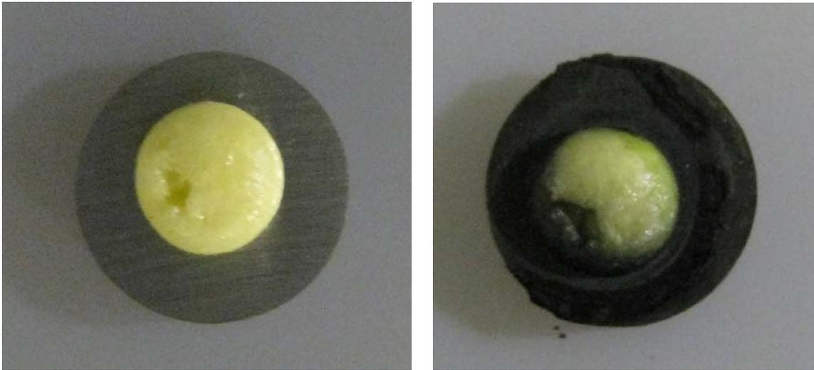
Figure 1. Corrosion coupon before and after 1 day exposure at 25°C.
