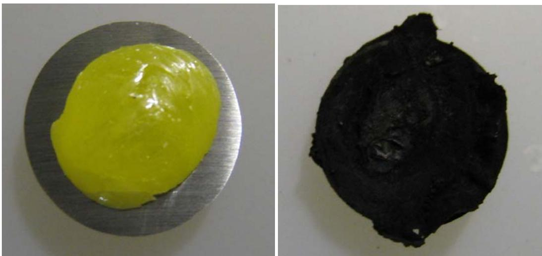
Figure 10. Corrosion coupon before and after 1 day exposure at 80°C.
