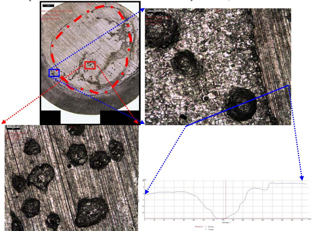
Figure 9. IFM data for coupon contacted with sulfur for 5 days at 25°C, without film, appearance of the surface and a line profile.
