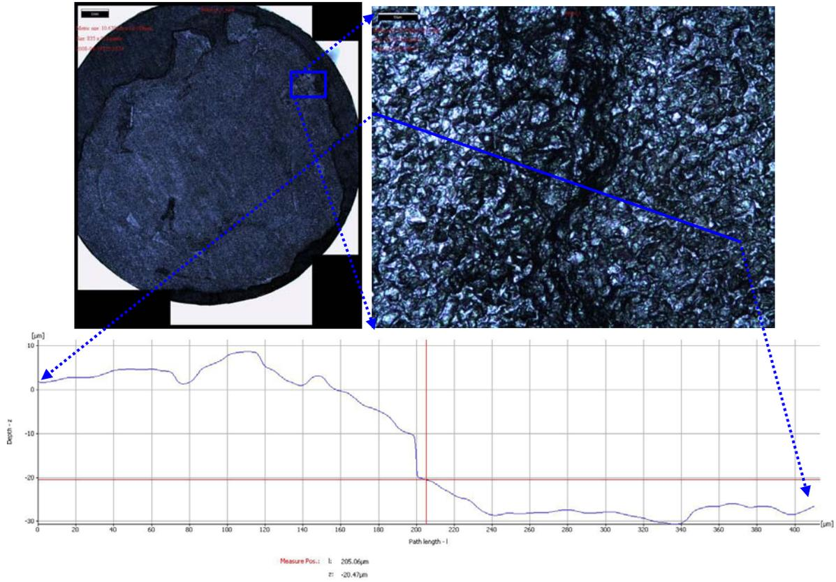
Figure 17. IFM data for coupon contacted with sulfur for 5 days at 80°C, without film, appearance of the surface and a line profile.
