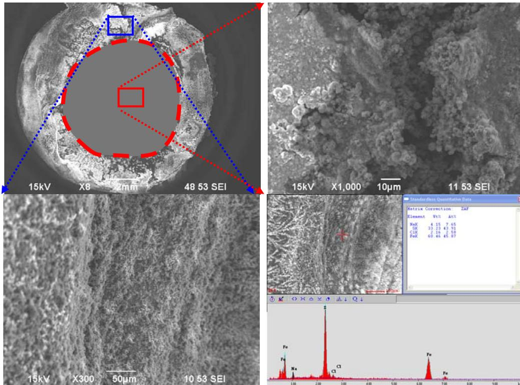
Figure 15. Corrosion coupon contacted with elemental sulfur for 4 days at 80°C, with film.
