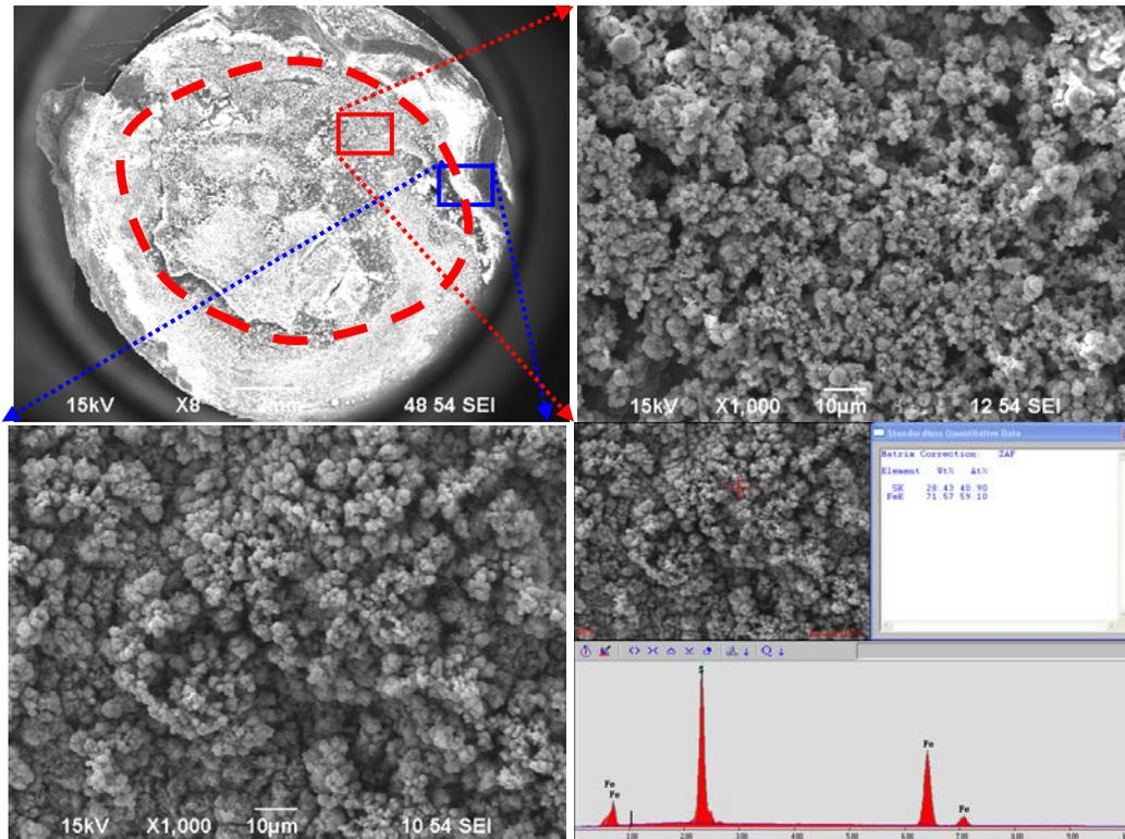
Figure 13. Corrosion coupon contacted with elemental sulfur for 1 day at 80°C, with film
