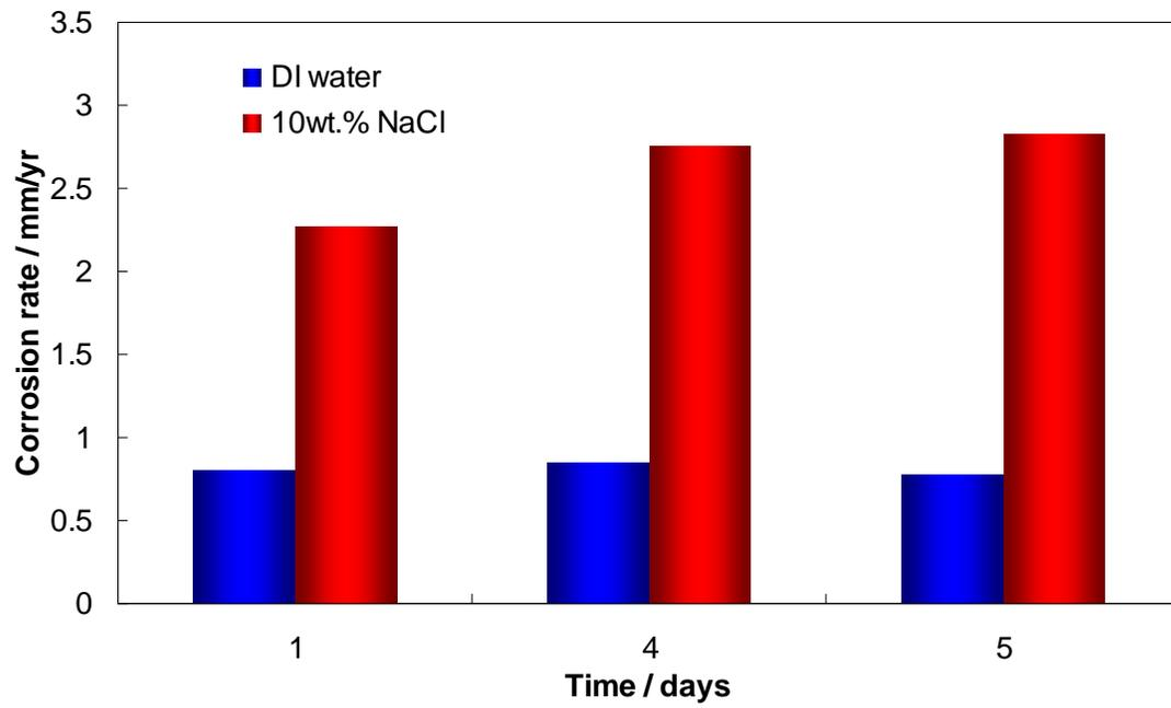
Figure 19. Comparisons of general corrosion between salt free and 10 wt.% NaCl conditions at 25°C.
