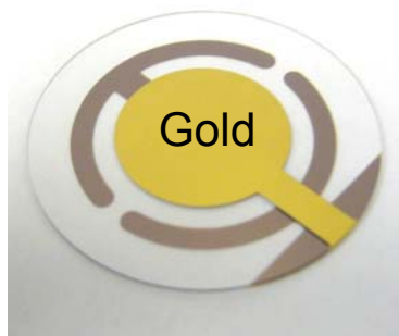
Figure 1. Quartz crystal microbalance and gold and iron coated quartz crystals
