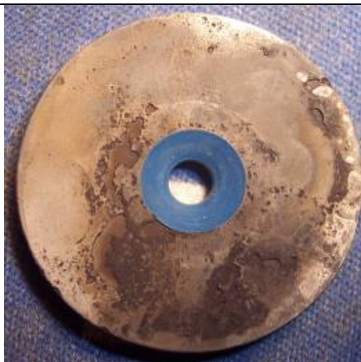
Scan of the coupon surface after removal of the corrosion product layer
