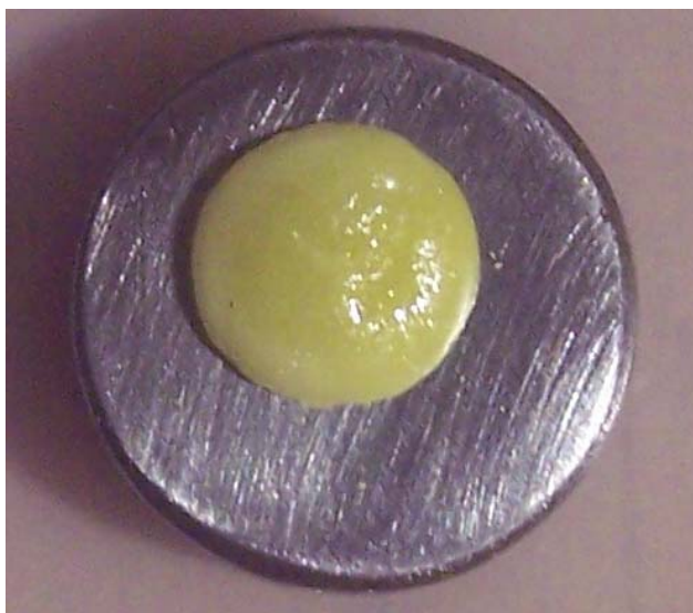
FIGURE 2 – Elemental sulfur deposited on the surface of a corrosion coupon before exposure.
