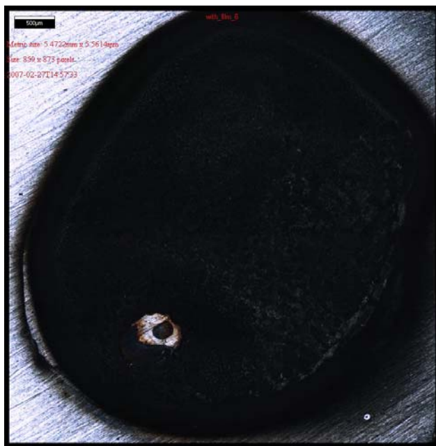
FIGURE 3 – The overall surface of a corrosion coupon after exposure to elemental sulfur (25°C, 3 days).
