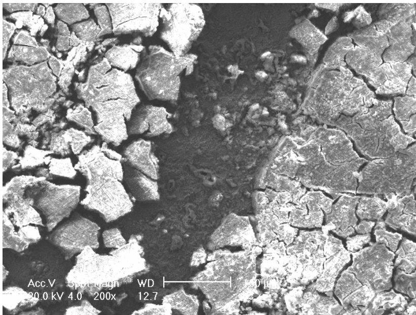
Figure 25. Experiment 3: Surface features of small UNS C1018 WL coupon from multiphase flow. SEM at 200X magnification shows multiple layers. (60°C, 0.77 MPa CO 2 , pH 6, H 2 S gas phase concentration = 120 \pm 10 ppm, 25 day exposure).
