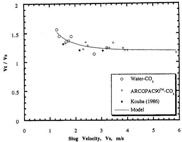
Fig. 2 Modeled variation of slug translational velocity with slug velocity
