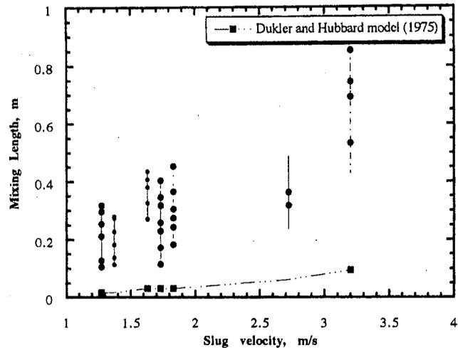
Fig. 4 Variation of mixing length with slug velocity water-CO<sub>2</sub> slug system
