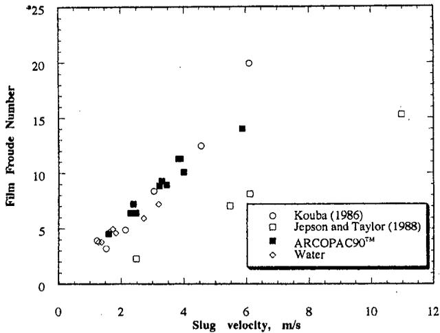
Fig. 3 Variation of film Froude number with slug velocity
