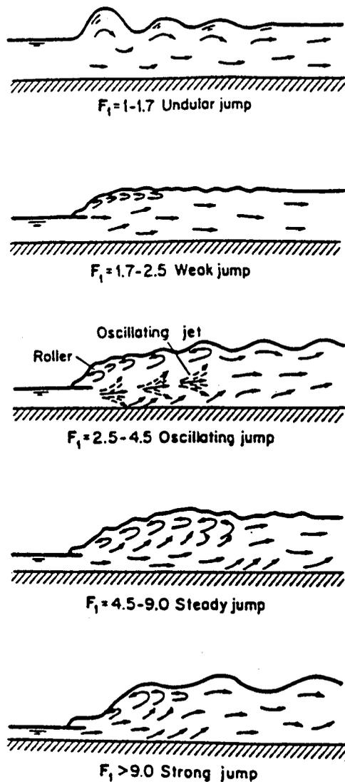
Fig. 1 Types of hydraulic jumps
