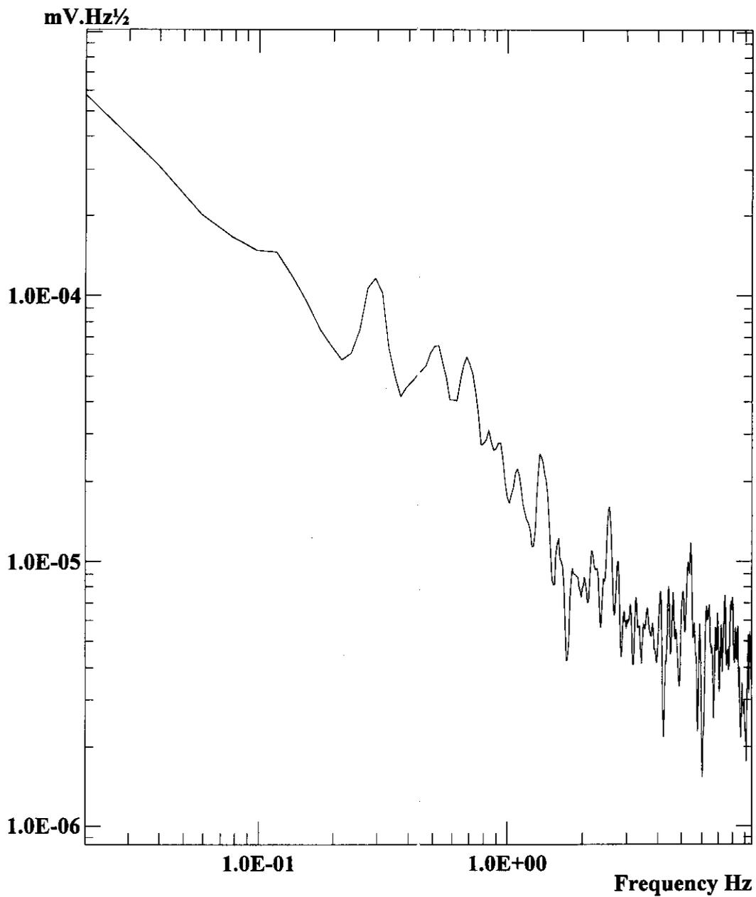
**Figure 6. Potential amplitude spectrum for 1.1 m/s full pipe flow.
