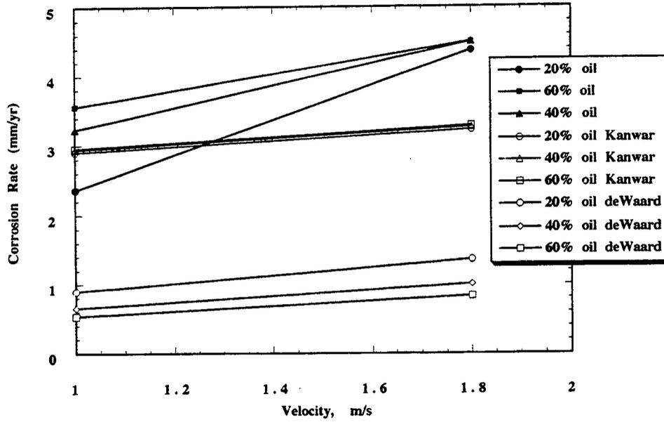
Figure 9 : Corrosion rate vs velocity using 96 cp oil
