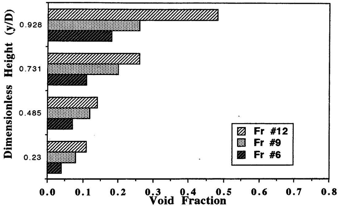
Figure 7a: Void fraction across the pipe Diameter
