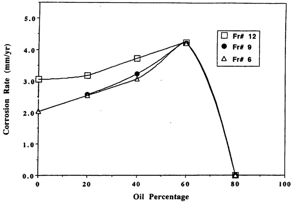
Figure 5: Corrosion rate vs oil percentage
