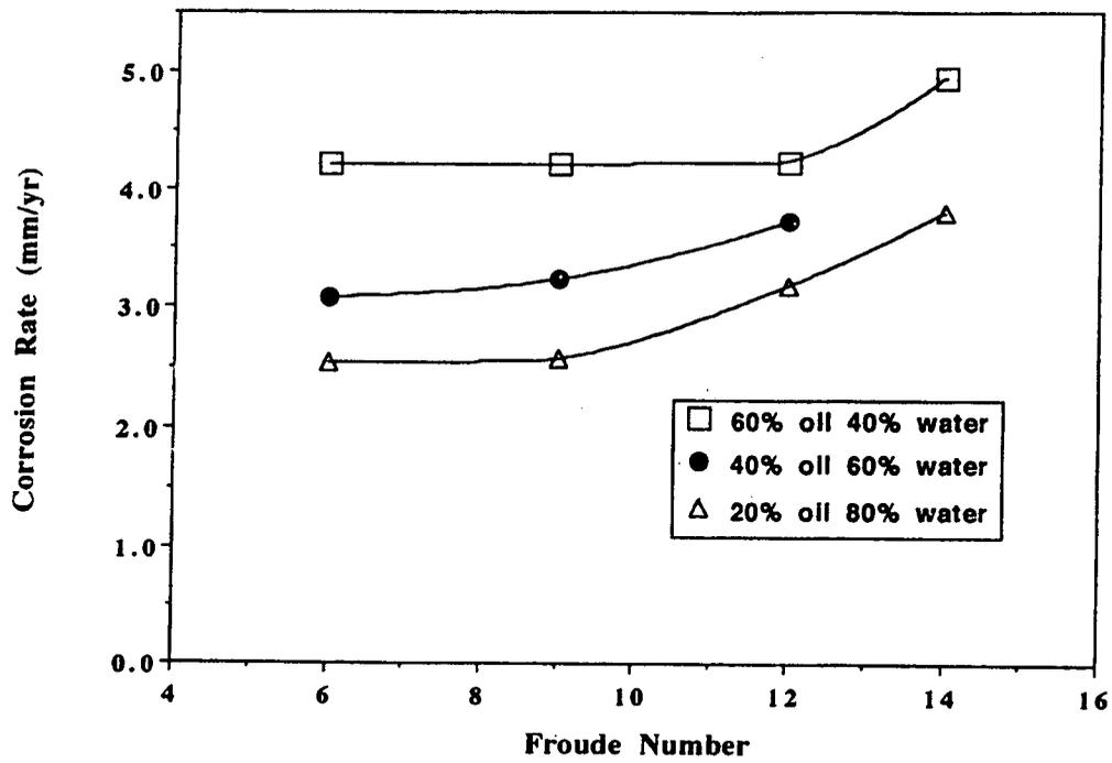
Figure 6: Corrosion rate vs Froude number
