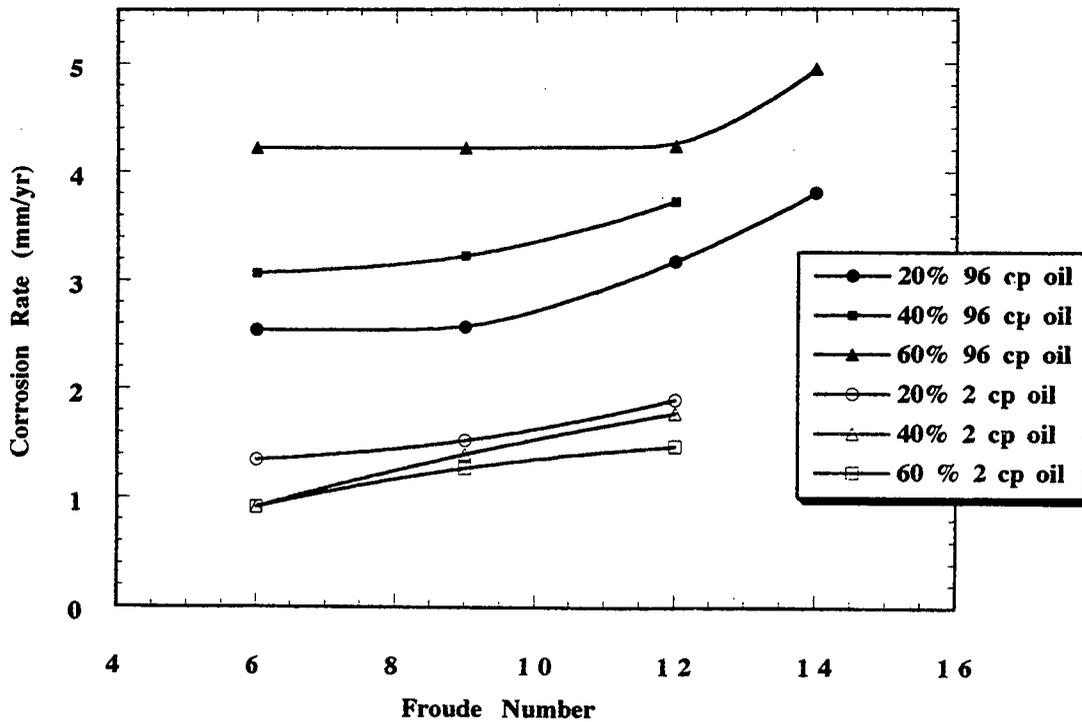
Figure 10: Corrosion rate vs Froude number
