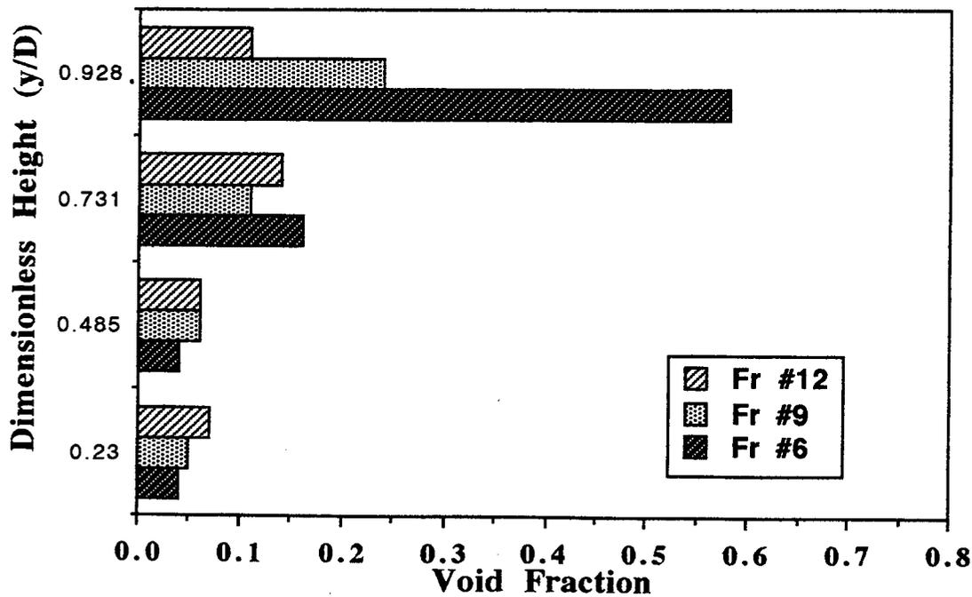
Figure 7d: Void fraction across the pipe diameter
