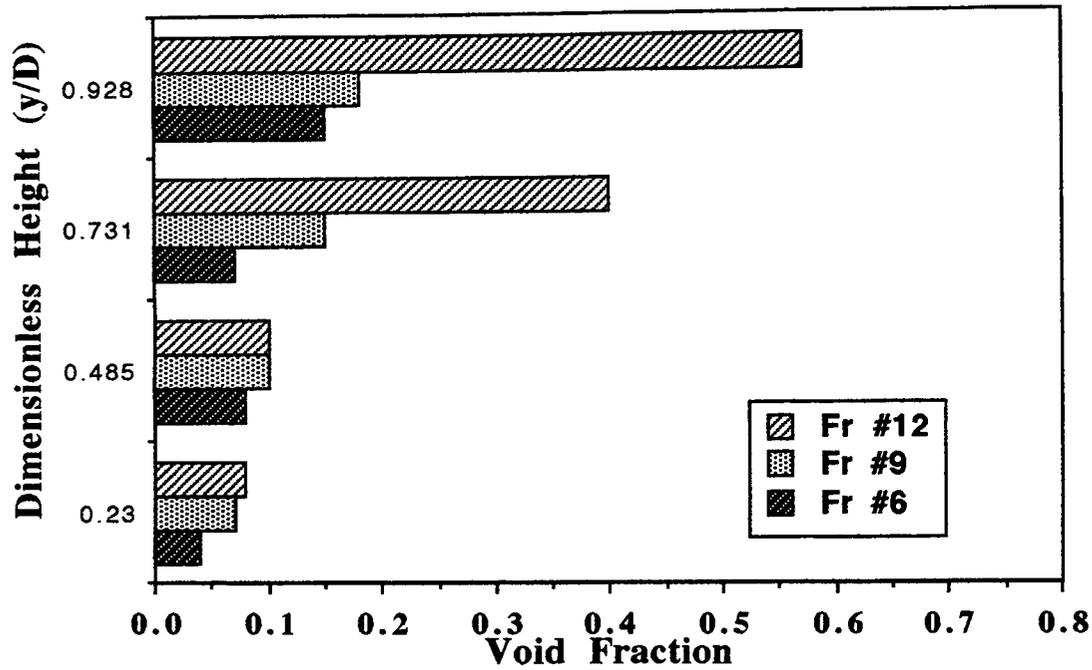
Figure 7c: Void fraction across the pipe diameter
