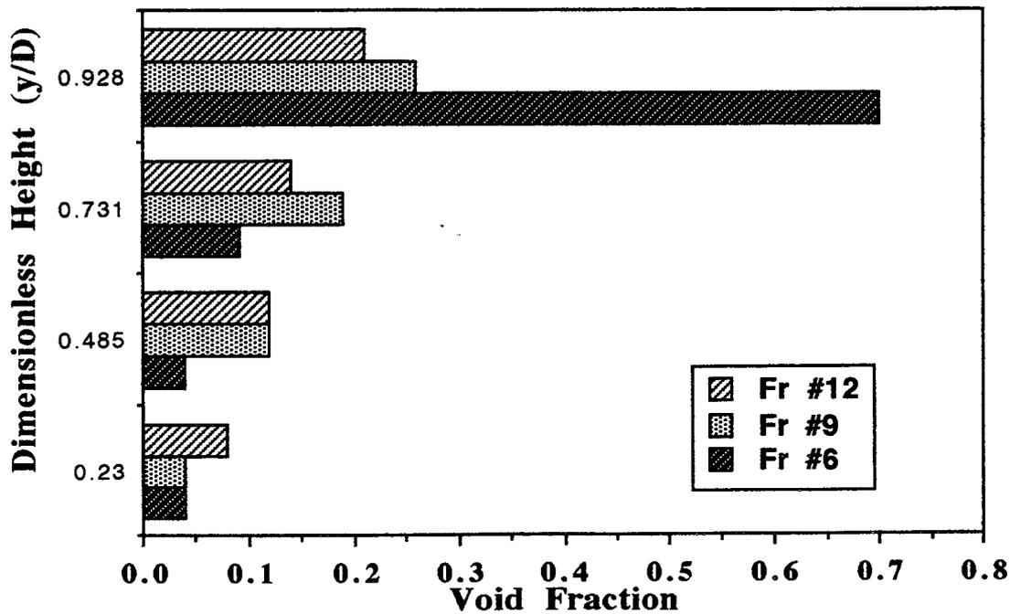
Figure 7b: Void fraction across the pipe diameter
