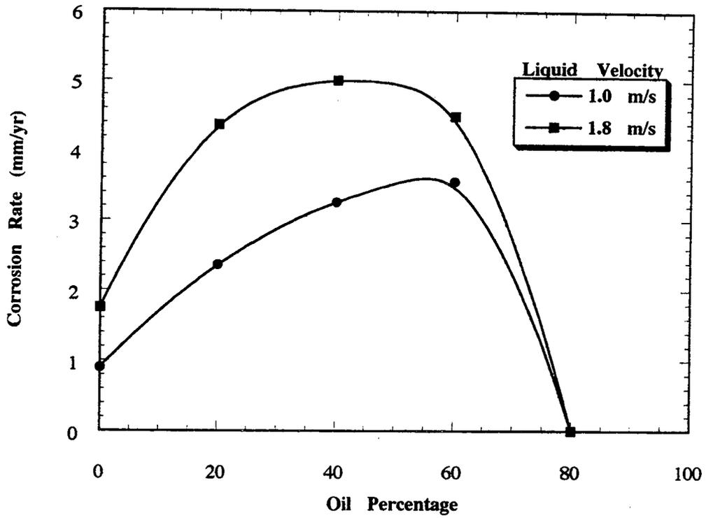
Figure 4: Effect of oil percentage on corrosion rate for full pipe flow
