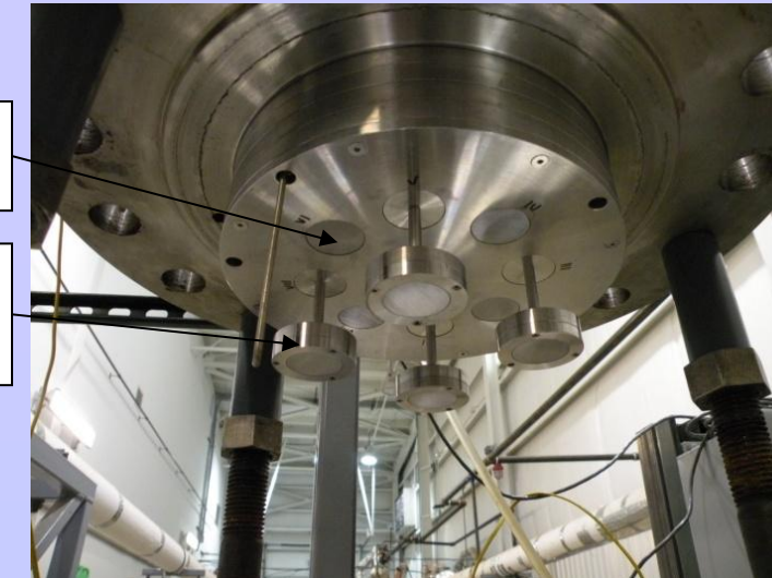
Coupons holder setup for top of line samples
