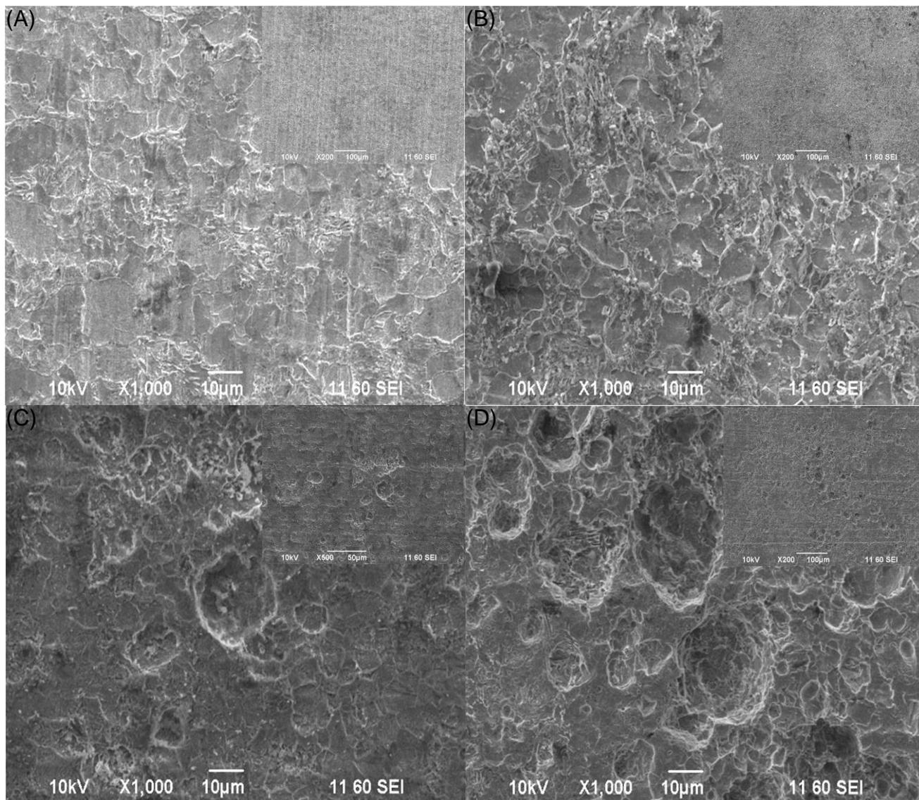
**Figure 2. SEM pit images of cleaned X65 coupons after hydrotest in natural seawater: (A) no spiking at 37°C after 90 days, (B) No SRB spiking at 22°C after 90 days, (C) spiked with  $10^6$  cells/ml SRB at 37°C after 90 days, (D) spiked with  $10^6$  cells/ml SRB at 22°C after 90 days. The smaller inserted SEM images inside (A, B, D) all have a scale bar of 100 microns. For (C), it is 50 microns.**
