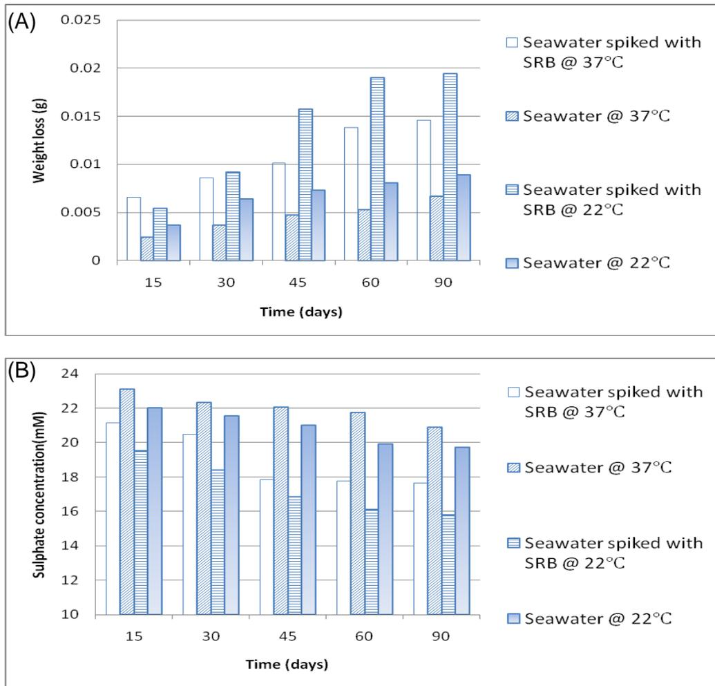
**Figure 4. (A) Weight loss data for 90-day coupons, and (B) residual sulfate concentration after 90 days.**
