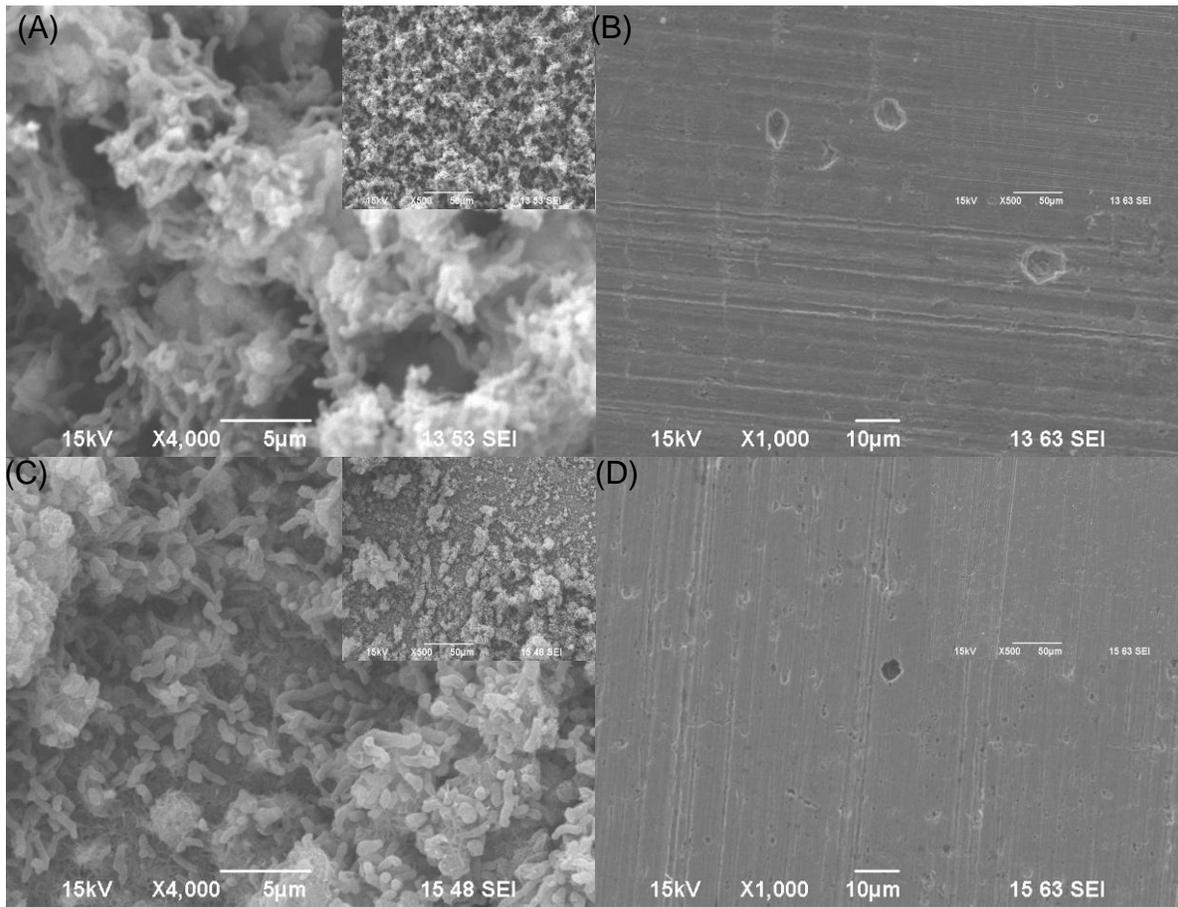
**Figure 5. SEM biofilm images and pit images (after biofilm removal) on coupons. Coupons were from 30-day simulated hydrotest using enriched artificial seawater spiked with  $10^6$  cells/ml SRB at 22°C (A and B) and 37°C (C and D).**
