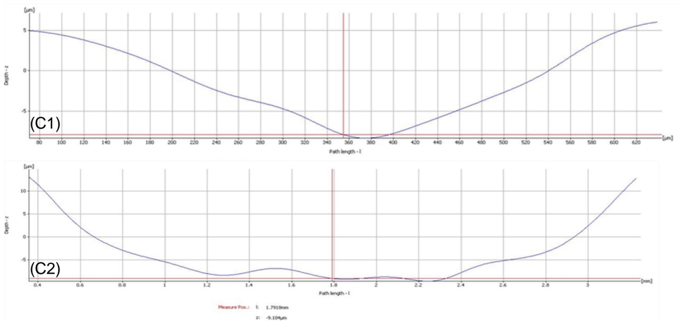
**Figure 9. Profilometer analysis of a coupon surface: (A1) Overview, (B1) a selected spot; (C1) depth profile of the spot. Coupon 1 (corresponding to A1, B1, C1) was the same as the one used for Figure 8B. Profilometer analysis of a coupon surface: (A2) Overview, (B2) a selected spot; (C2) depth profile of the spot. Coupon 2 was the same as the one used for Figure 8D.**
