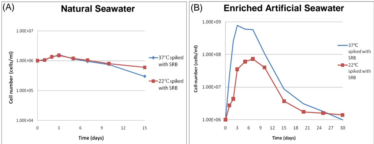
**Figure 3. Planktonic cell counts in natural seawater spiked with  $10^6$  cells/ml SRB (A), and in enriched artificial seawater spiked with  $10^6$  cells/ml SRB (B).**
