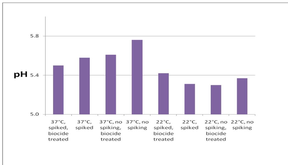
**Figure 6. Water phase pH values for vials after 15 days with X65 coupons in a simulated pipeline fluid (oil mixed with natural seawater) saturated with 1 bar CO<sub>2</sub> in the headspace.**
