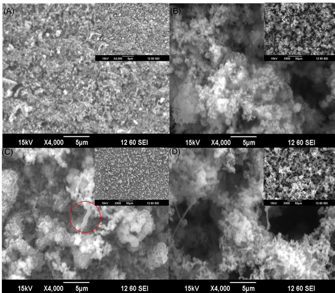
**Figure 1. SEM biofilm images on X65 coupon surfaces. Coupons were from 90-day simulated hydrotest in natural seawater: (A) without SRB spiking at 37°C, (B) without SRB spiking at 22°C, (C) spiked with  $10^6$  cells/ml SRB at 37°C, and (D) spiked with  $10^6$  cells/ml SRB at 22°C.**
