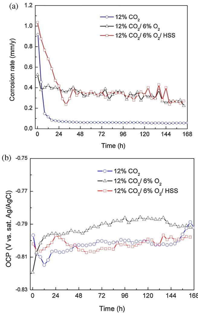
**Fig. 2.** Variations of (a) corrosion rate and (b) OCP of carbon steel in MEA systems with different test conditions.
