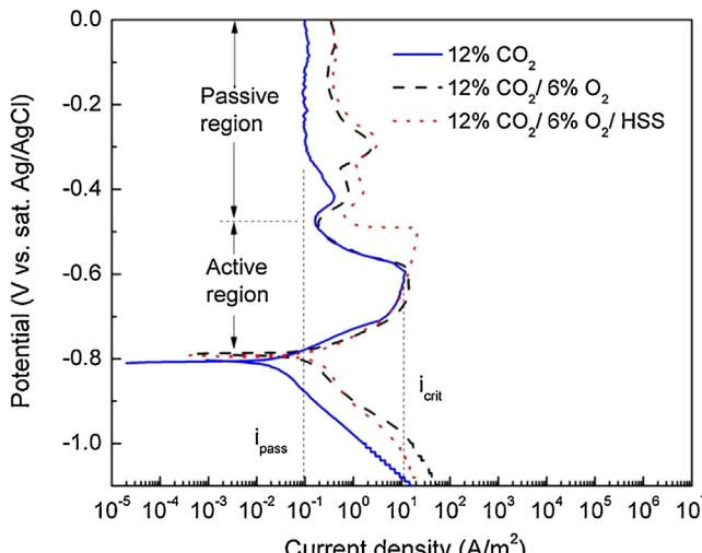
**Fig. 5.** Polarization curves of carbon steel in MEA systems with O<sub>2</sub> and HSS (after 7-day exposure).
