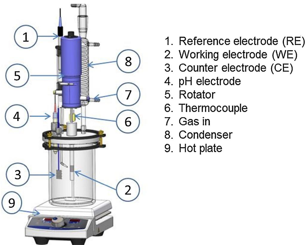
**Fig. 1.** Schematic of experimental setup for MEA corrosion tests.
