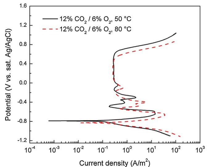
**Fig. 11.** Effect of temperature on the polarization behavior of carbon steel under MEA/CO<sub>2</sub>/O<sub>2</sub> condition (after 7-day exposure).
