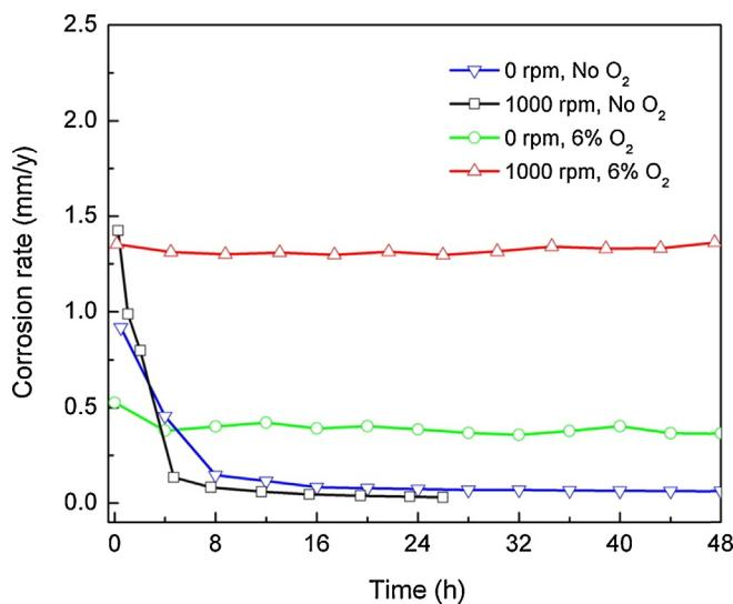
**Fig. 8.** Effect of flow on the corrosion rate of carbon steel with time under different conditions.
