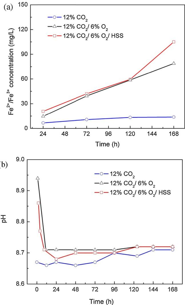
**Fig. 3.** Variations of (a) Fe<sup>2+</sup>/Fe<sup>3+</sup> concentrations and (b) MEA solution pH with different test conditions.
