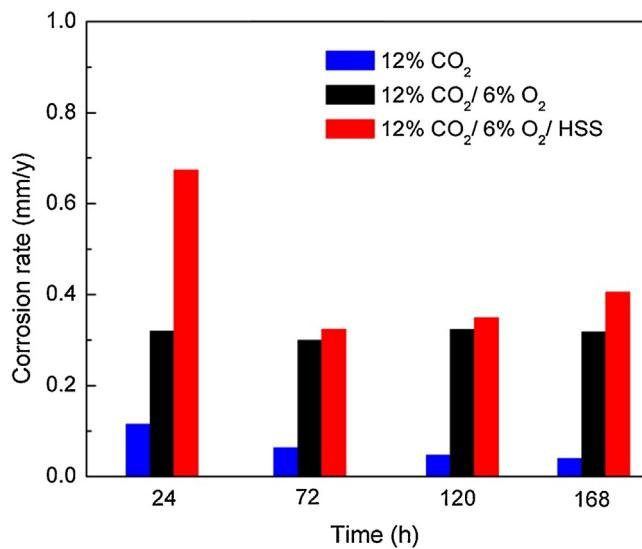
**Fig. 4.** Variation of corrosion rates of carbon steel with time measured from weight loss method in MEA systems.
