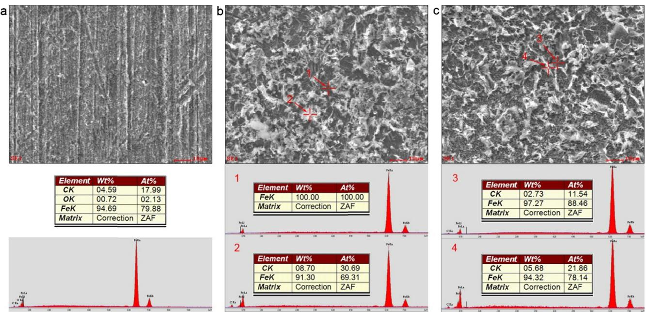
**Fig. 6.** SEM images and EDS spectra of the corroded surface of the samples after 7-day exposure: (a) MEA/CO<sub>2</sub>, (b) MEA/CO<sub>2</sub>/O<sub>2</sub>, (c) MEA/CO<sub>2</sub>/O<sub>2</sub>/HSS.
