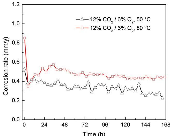
**Fig. 10.** Variations of corrosion rate in MEA/CO<sub>2</sub>/O<sub>2</sub> system with different temperatures.
