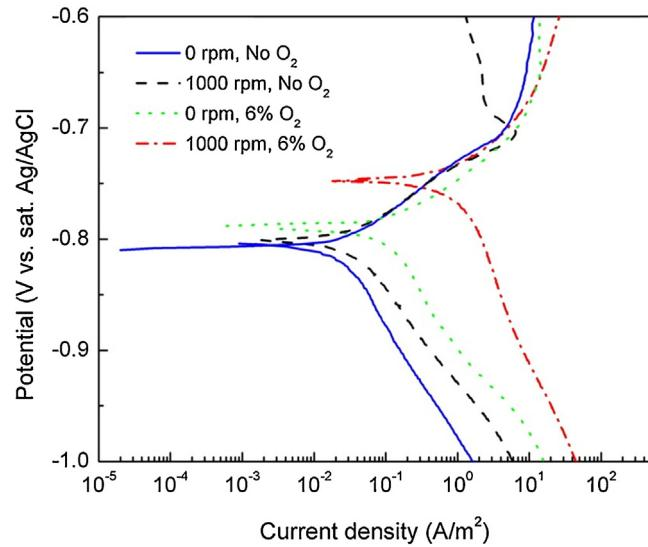
**Fig. 9.** Effect of flow on the polarization behavior of carbon steel under different conditions (after 7-day exposure).
