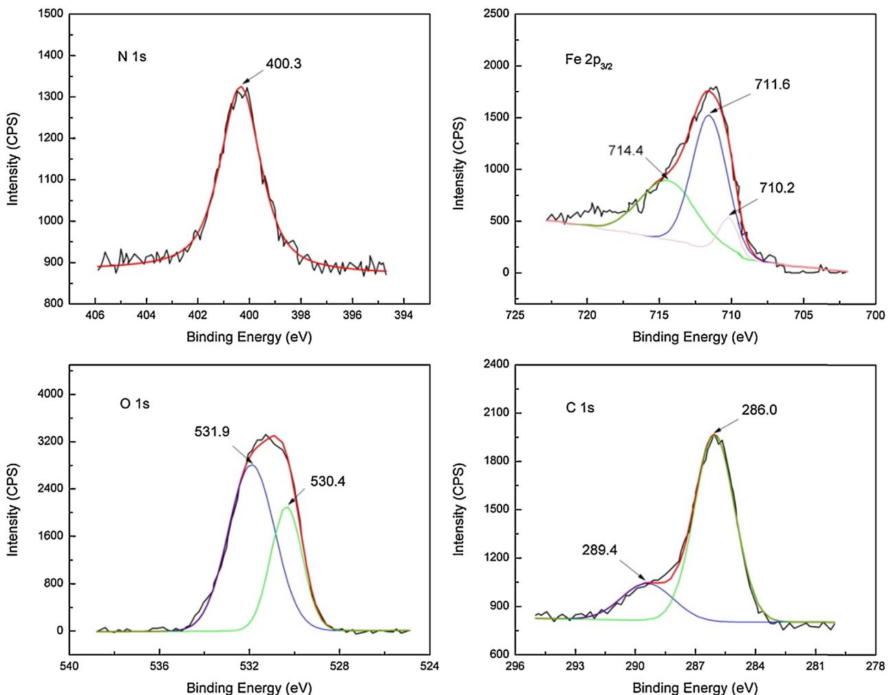
**Fig. 7.** XPS spectra of carbon steel exposed to MEA/CO<sub>2</sub> system for 7 days.
