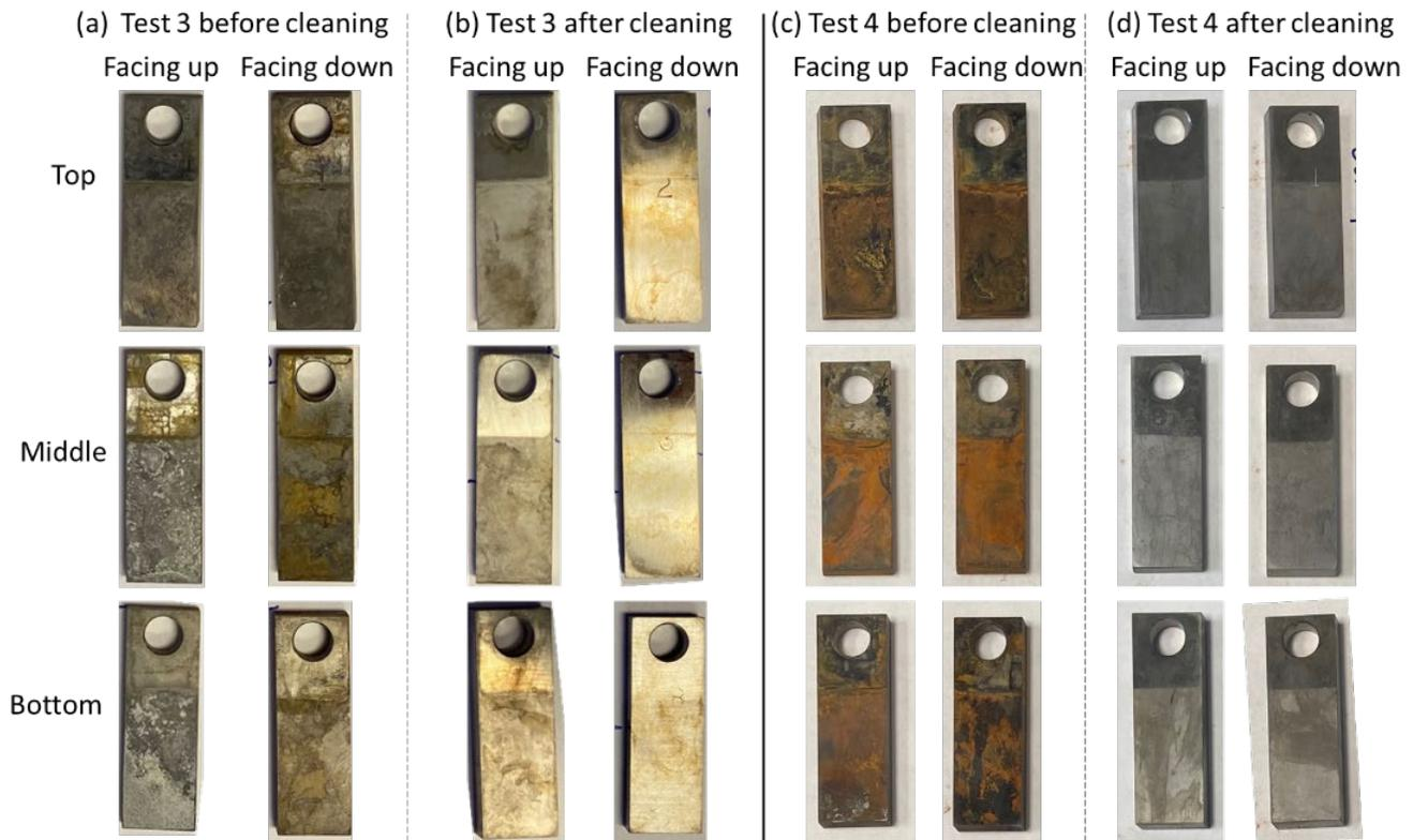
**Figure 5: Photos of Test 3 and Test 4 samples before and after cleaning. “Facing up” and “facing down” indicate the two sides of the same sample. “Top”, “Middle”, and “Bottom” are the locations of samples inside the autoclave during test.**
