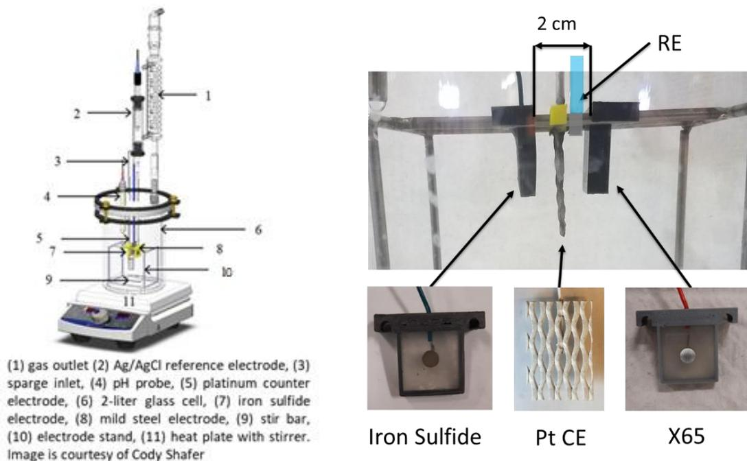
**Figure 1. Overview of the experimental setup (left), and image of the electrochemical cell (right)**
