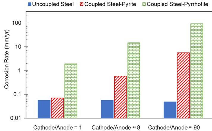
**Figure 7. The effect of cathode to anode surface area ratio on corrosion rates of uncoupled and coupled X65 mild steel at 30 °C, 1 wt.% NaCl, pH 5**
