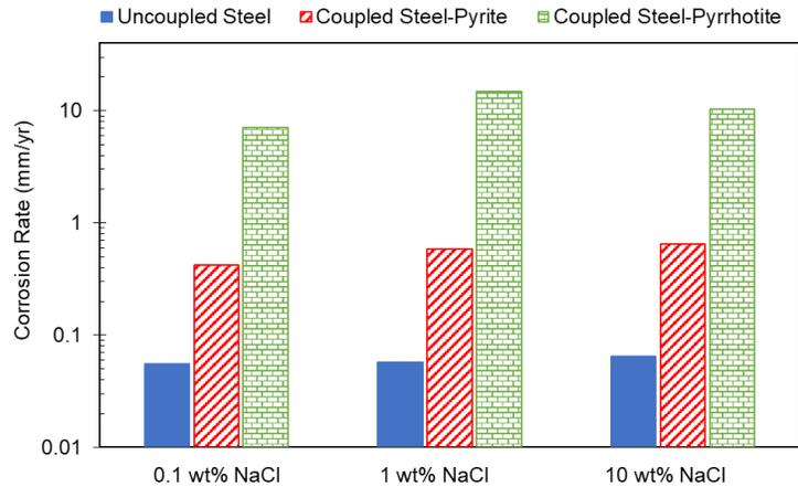
**Figure 11. The effect of salt concentration on corrosion rates of uncoupled and coupled steel at 30 °C, pH 5, cathode/anode surface area ratio = 8.**
