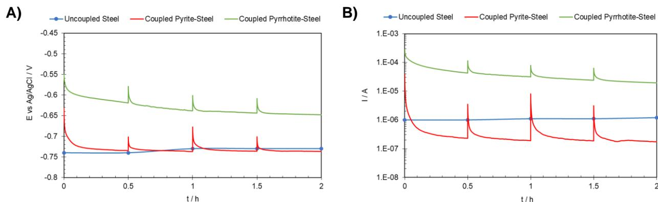
**Figure 2. A) potential, B) current of steel when coupled to pyrrhotite and pyrite at 30 °C, 1 wt.% NaCl, pH 5, cathode/anode ratio = 1**
