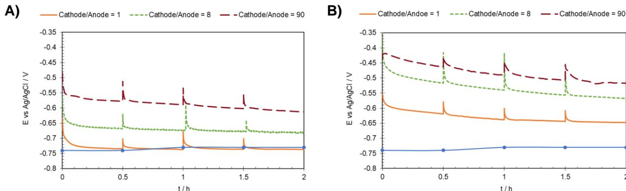
**Figure 5. The effect of cathode to anode surface ratio on the galvanic potential of steel when coupled to A) pyrite, and B) pyrrhotite at 30 °C, 1 wt.% NaCl, and pH 5. The solid blue line shows the open circuit potential of uncoupled steel.**
