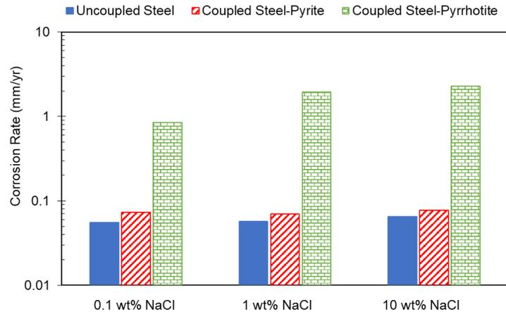
**Figure 9. The effect of salt concentration on corrosion rates of uncoupled and coupled steel at 30 °C, pH 5, cathode/anode surface area ratio = 1**
