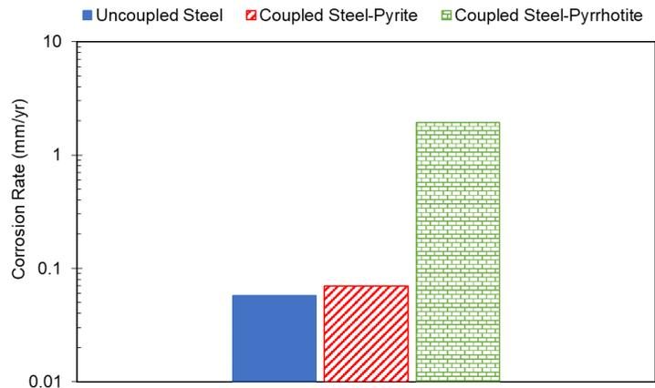
**Figure 4. Calculated corrosion rates of uncoupled and coupled X65 mild steel at 30 °C, 1 wt.% NaCl, pH 5, cathode/anode surface area ratio = 1.**
