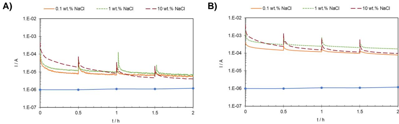
**Figure 10. The effect of salt concentration on the galvanic current of steel when coupled to A) pyrite, and B) pyrrhotite at 30 °C, pH 5, and cathode/anode surface area ratio = 8. The solid blue line shows the corrosion current of uncoupled steel.**
