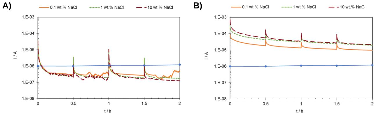
**Figure 8. The effect of salt concentration on the galvanic current of steel when coupled to A) pyrite, and B) pyrrhotite at 30 °C, pH 5, and cathode/anode surface area ratio = 1. The solid blue line shows the corrosion current of uncoupled steel.**
