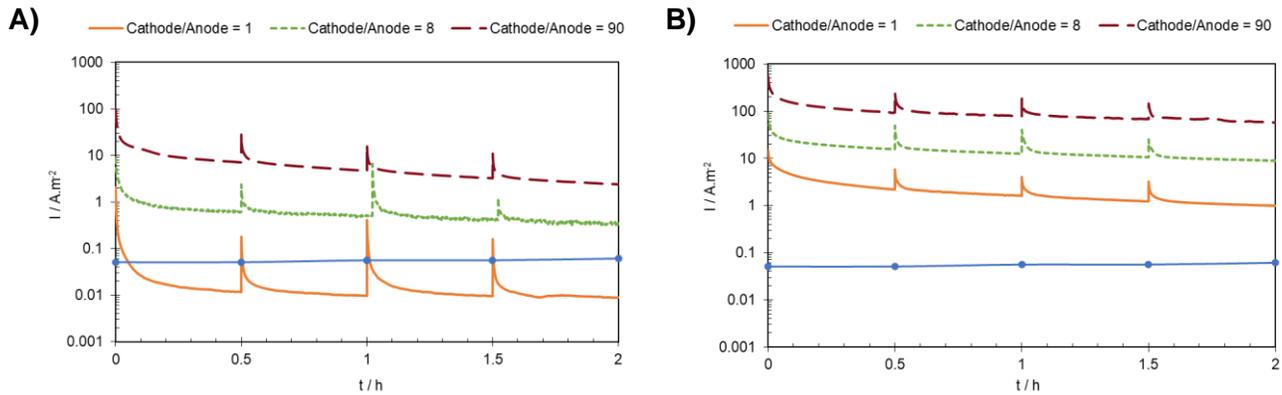
**Figure 6. The effect of cathode to anode surface area ratio on the galvanic current of steel when coupled to A) pyrite, and B) pyrrhotite at 30 °C, 1 wt.% NaCl, and pH 5. The solid blue line shows the corrosion current of uncoupled steel.**
