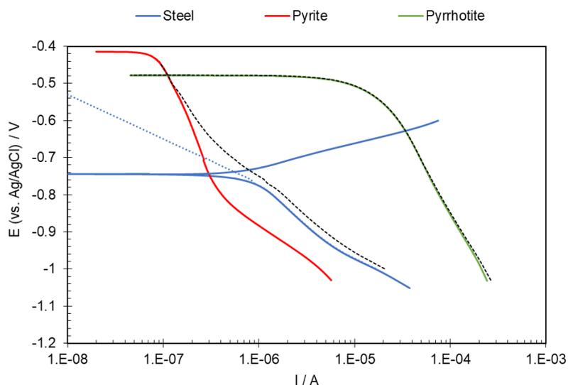
**Figure 3. Potentiodynamic sweeps on X65 mild steel, pyrite and pyrrhotite at 30 °C, 1 wt.% NaCl, pH 5, and cathode/anode surface area ratio = 1 (black dotted lines = total cathodic currents, and blue dotted line = calculated cathodic current on steel).**
