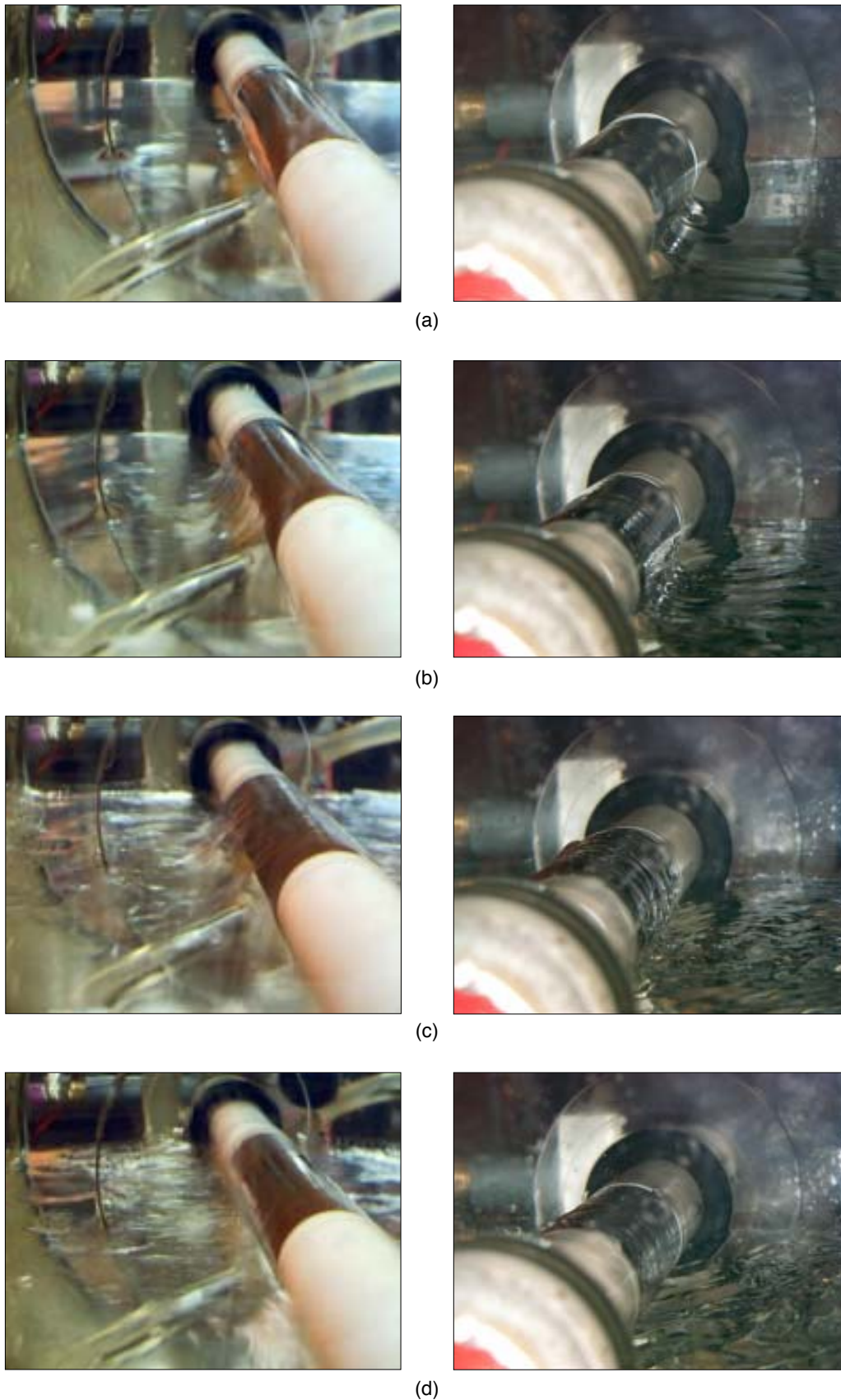
FIGURE 3. Images of the rotating cylinder and the water/hydrocarbon interface at 30% water cut and various speeds: (a) stationary electrode, (b) 500 rpm, (c) 1,000 rpm, and (d) 1,500 rpm.
