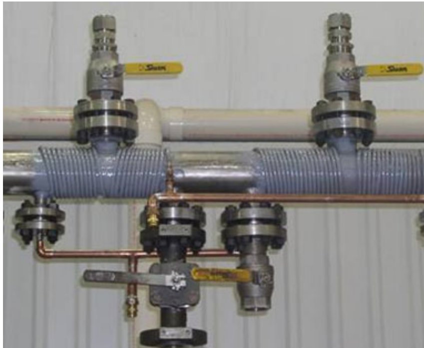
Figure 3 - Test section of the H 2 S loop Only the bottom ports were used in this study
