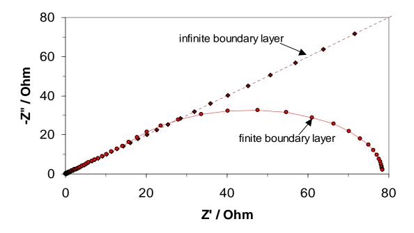
Figure 8. Comparison between calculated electrochemical impedance of H<sup>+</sup> ions for a finite-thickness diffusion boundary layer,  $\delta_{B.L.}$ =0.003m and infinite-thickness diffusion boundary layer, also known as Warburg impedance, for T=20°C,  $[H^+]_{bulk}$ =1×10<sup>-5</sup> mol/liter
