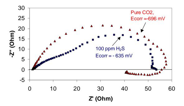
Figure 6. Effect of 100 ppm gaseous  $H_2S$  on the Nyquist impedance diagram at steady state condition for carbon steel X65 in pH5 saturated CO<sub>2</sub> solution of water + 3%NaCl, p=1 bar, t=20<sup>o</sup>C,  $\omega$ =1000rpm at corrosion potential (vs. Ag/AgCl).
