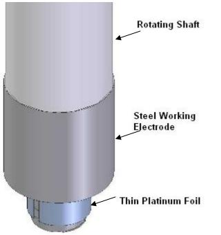
Figure 12. Schematics of old design specimen holder section of rotating shaft
