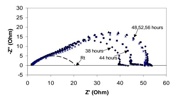
Figure 5. Magnification of the above Figure 4; effect of immersion time (after 40 hours) on the Nyquist impedance diagram of carbon steel X65 in pH5 saturated CO<sub>2</sub> solution with 100 ppm gaseous H<sub>2</sub>S, water + 3%NaCl, p=1 bar, t= $20^{\circ}$ C,  $\omega$ = 1000rpm at corrosion potential (vs. Ag/AgCl)
