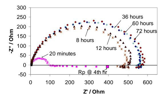
Figure 15. Effect of immersion time on Nyquist impedance diagram of carbon steel X65 in pH 5 saturated CO<sub>2</sub> solution with 340 ppm gaseous H<sub>2</sub>S, water + 3% NaCl, p = 1 bar, t =  $20^{\circ}$ C,  $\omega = 1000$  rpm at corrosion potential.
