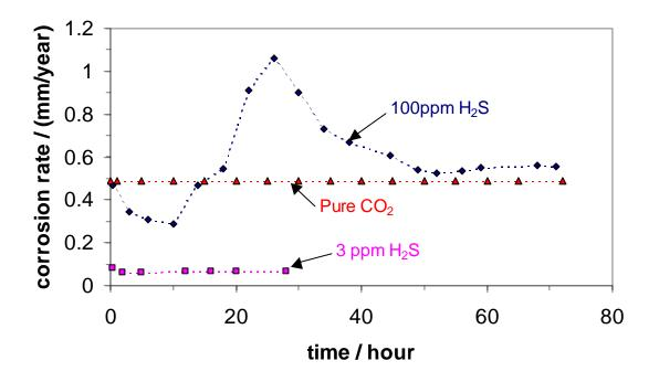
Figure 7. Effect of H<sub>2</sub>S gaseous concentration on the corrosion rate (measured by LPR) of carbon steel X65 in pH5 saturated CO<sub>2</sub> solution, water + 3%NaCl, p=1 bar,  $t=20^{0}$ C,  $\omega=1000$ rpm with respect to immersion time.
