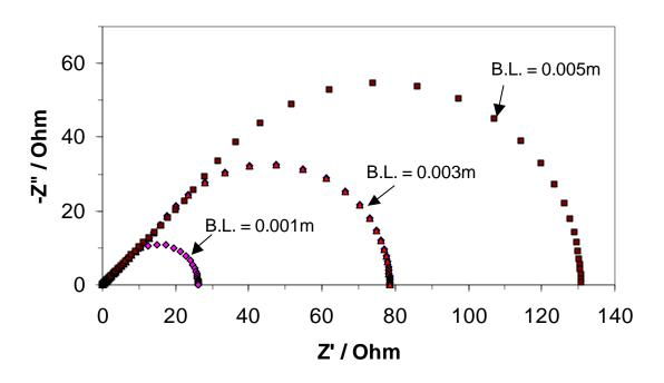
Figure 9. Effect of the thickness of diffusion boundary layer on the characteristics of electrochemical impedance of H<sup>+</sup> ions for T=20°C,  $[H^+]_{bulk}$ =1×10<sup>-5</sup> mol/liter
