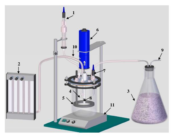
Figure 1. Schematic of the experimental test cell: 1-Ag/AgCl reference electrode, 2-gas rotameter,  $3-H_2S$  scrubber (gas absorbent), 4-Luggin capillary, 5-graphite counter electrode, 6-rotator, 7-pH electrode, 8-working electrode, 9-gas out, 10-gas in, 11-temperature control unit/stirrer.
