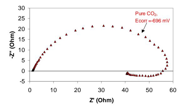
Figure 2. Nyquist impedance diagram for carbon steel X65 in pH5 saturated CO<sub>2</sub> solution of water + 3%NaCl, p=1 bar, t= $20^{\circ}$ C,  $\omega$ =1000rpm at corrosion potential (vs.Ag/AgCl).
