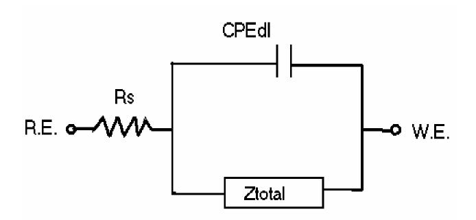
Figure 10. The equivalent circuit of the EIS model. Rs = solution resistance,  $CPEdl = constant phase elements describing double layer capacitance, <math>Z_{total} = total$  impedance, R.E. = reference electrode, W.E. = working electrode.
