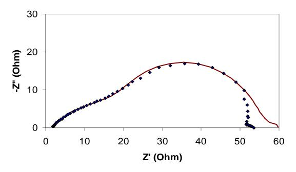
Figure 11. Comparison between experimental data (points) and model prediction (line) for 100 ppm gaseous H<sub>2</sub>S in CO<sub>2</sub>, water + 3%NaCl, p=1 bar, t= $20^{0}$ C,  $\omega$ = 1000rpm at corrosion potential (vs. Ag/AgCl).
