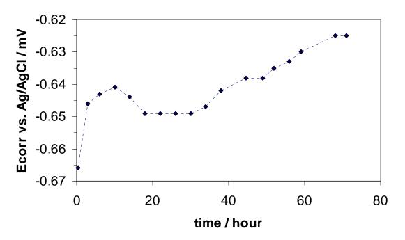
Figure 3. Corrosion potential with respect to immersion time for carbon steel X65 in pH5 saturated  $CO_2$  solution with100 ppm gaseous H<sub>2</sub>S in water +3%NaCl, p=1 bar, t=20<sup>o</sup>C,  $\omega$ =1000rpm.
