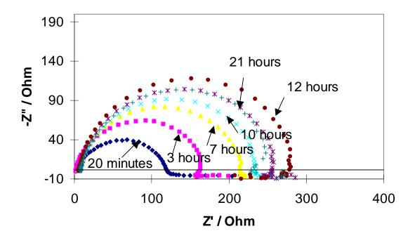
Figure 14. Effect of immersion time on Nyquist impedance diagram of carbon steel X65 in pH 5 saturated CO<sub>2</sub> solution with 100 ppm gaseous H<sub>2</sub>S, water + 3% NaCl, p = 1 bar, t =  $20^{\circ}$ C,  $\omega$  = 1000 rpm at corrosion potential.
