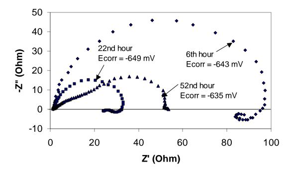
Figure 4. Effect of immersion time on the Nyquist impedance diagram of carbon steel X65 in pH5 saturated CO<sub>2</sub> solution with 100 ppm gaseous H<sub>2</sub>S, water + 3%NaCl, p=1 bar, t= $20^{\circ}$ C,  $\omega$ = 1000rpm at corrosion potential (vs. Ag/AgCl) during the same experiment.
