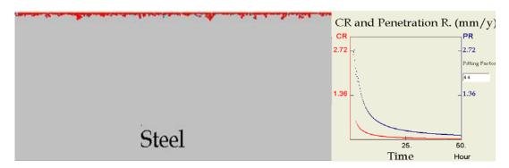
Figure 14. Surface morphology and the trend of the corresponding uniform corrosion rate (lower curve denoted CR) and localized penetration rate (upper curve denoted PR) as predicted by 2-D model at 50 ppm Fe<sup>2+</sup>, 0.54bar pCO<sub>2</sub>, 80 °C, pH 6.6, and 1m/s.
