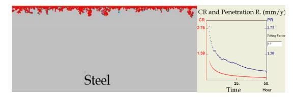
Figure 13. Surface morphology and the trend of the corresponding uniform corrosion rate (lower curve denoted CR) and localized penetration rate (upper curve denoted PR) as predicted by 2-D model at 30 ppm  $Fe^{2+}$ , 0.54bar pCO<sub>2</sub>, 80 °C, pH 6.6, and 1m/s.
