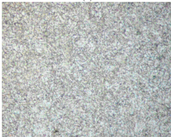
Figure 5. Microstructure of the X65 carbon steel a-b) longitudinal cut, c-d) transversal cut
