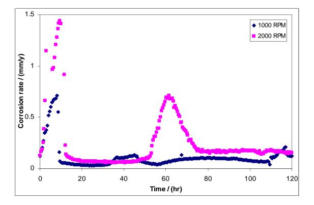
FIGURE 9 - Effect of coupon rotational speed on corrosion at 1000 and 2000 rpm.
