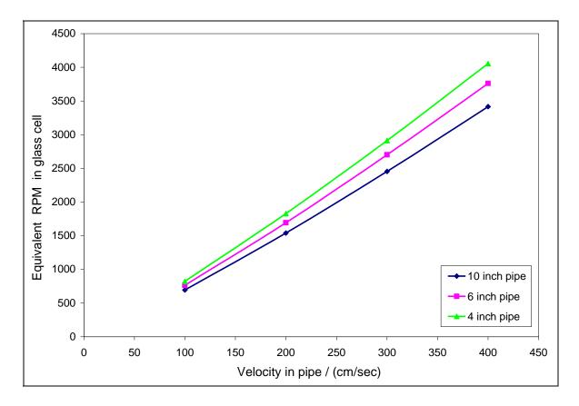
FIGURE 7 - Relation between rotational speed in glass cells and surface velocity for coupons in pipe flow.
