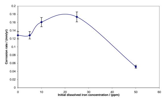
FIGURE 2 - Corrosion rate variation with the change in dissolved iron concentration.
