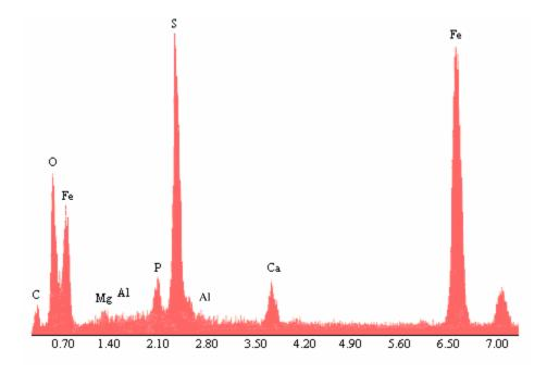
FIGURE 1 - EDS scan of metal coupon surface showing the presence of iron and sulfur
