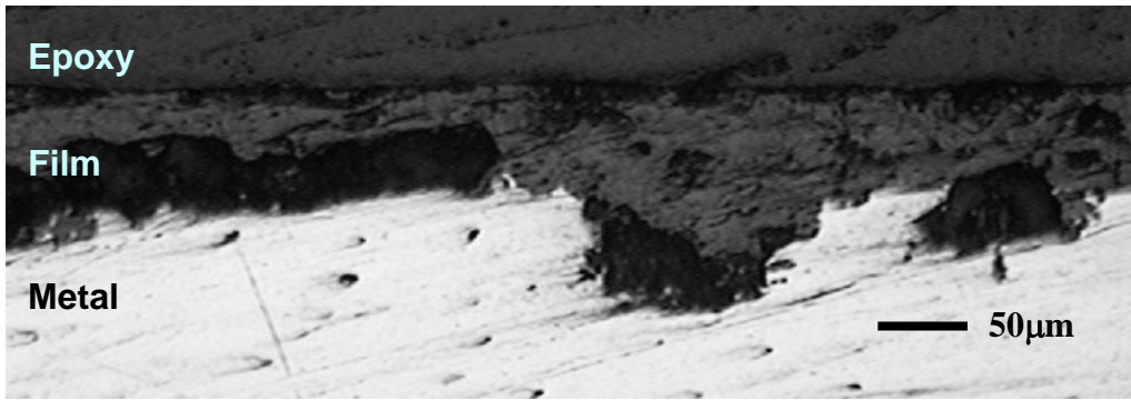
Figure 8. Experiment 1: X65(2), 30 day exposure to single phase flow, 60 to 125 μm film thickness, showing pitting. (100X metallurgical microscope, 60°C, 0.77 MPa CO 2 , pH 6, V sg = 3m/s, V sl = 1m/s, H 2 S gas phase concentration = 25 ± 10 ppm).
