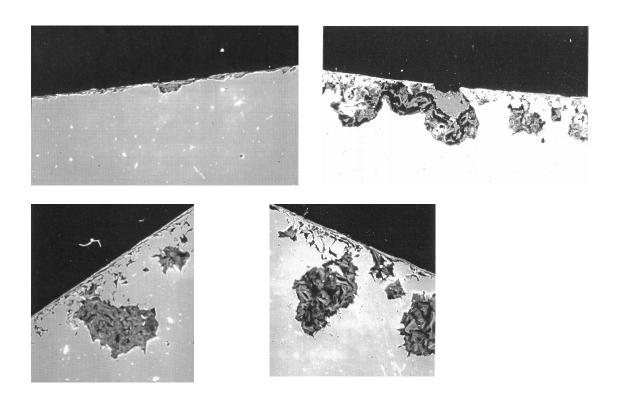
Figure 6. SEM images of the corroded steel surfaces taken from the study of CO2 corrosion in multiphase flow taken from the study by Nesic and Lunde<sup>(16)</sup>.
