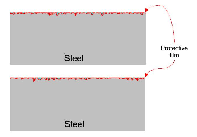
Figure 2. Two samples of the simulated metal surface morphology following rapid precipitation leading to a protective film and very little corrosion. Original Pots' algorithm was used.
