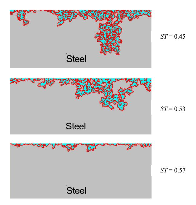
Figure 5. Three samples of a simulated metal surface morphology following moderate precipitation leading to a partially protective film and localized corrosion. The modified algorithm (equation 4) was used.
