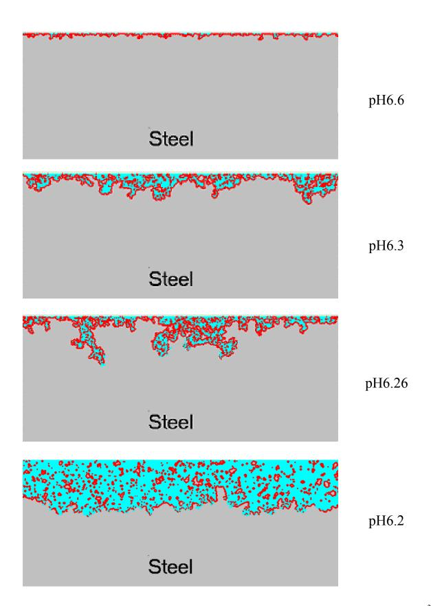
Figure 8. Predictions for the case of a 1%NaCl solution, at T = 80°C,  $P_{CO2} = 0.52$ bar, Ptotal = 1bar,  $C_{Fe}^{2+} = 100$ ppm., v=1 m/s.
