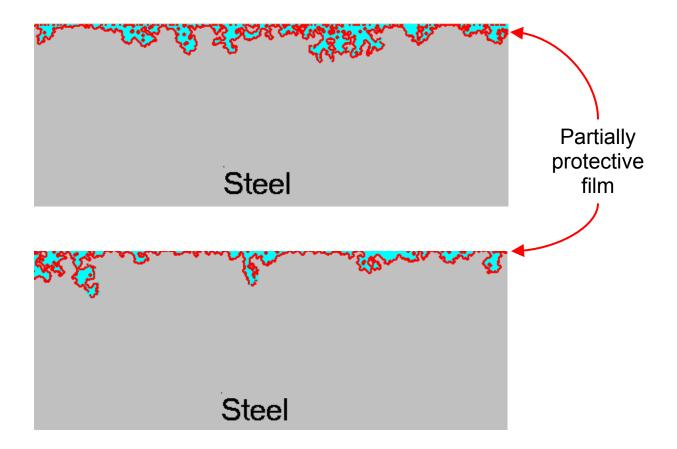
Figure 4. Two samples of simulated metal surface morphology following moderate precipitation leading to a partially protective film and localized corrosion. Original Pots' algorithm was used.
