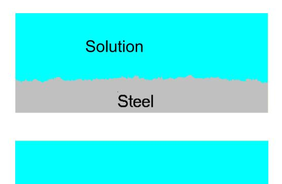
Figure 1. Two samples of simulated metal surface morphology following rapid uniform corrosion without any film precipitation. Original Pots'(14) algorithm was used.
