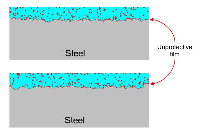
Figure 3. Two samples of simulated metal surface morphology following slow precipitation leading to an unprotective film and a moderate corrosion rate. Original Pots'(14) algorithm was used.
