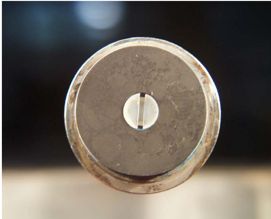
Figure 11: Corrosion product layer – Top of the line T=70 C, Low condensation rate, V_{\text{gaz}}=5 m/s, HAc=171ppm
