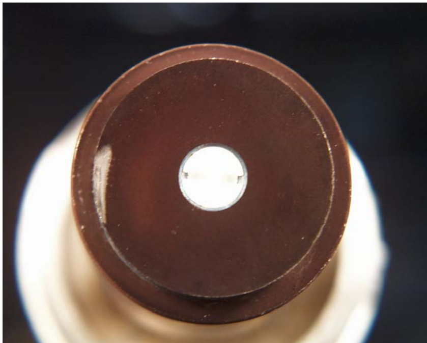
Figure 14: Corrosion product layer – Bottom of the line T=70 C, High condensation rate, V_{\text{gaz}}=5 m/s, HAc=171ppm
