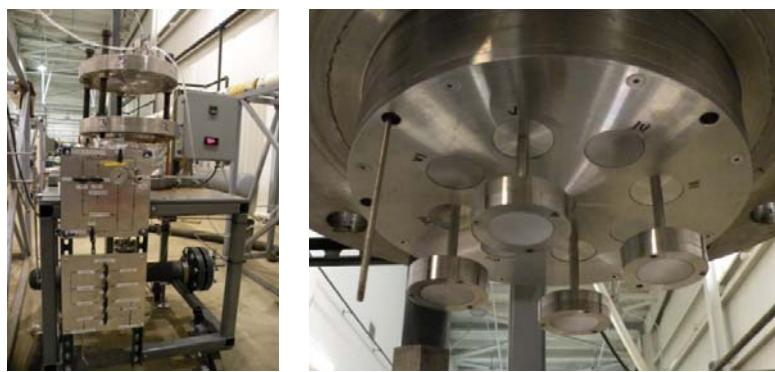
Figure 3: 20L autoclave setup (left) and details of the sample holder (right)
