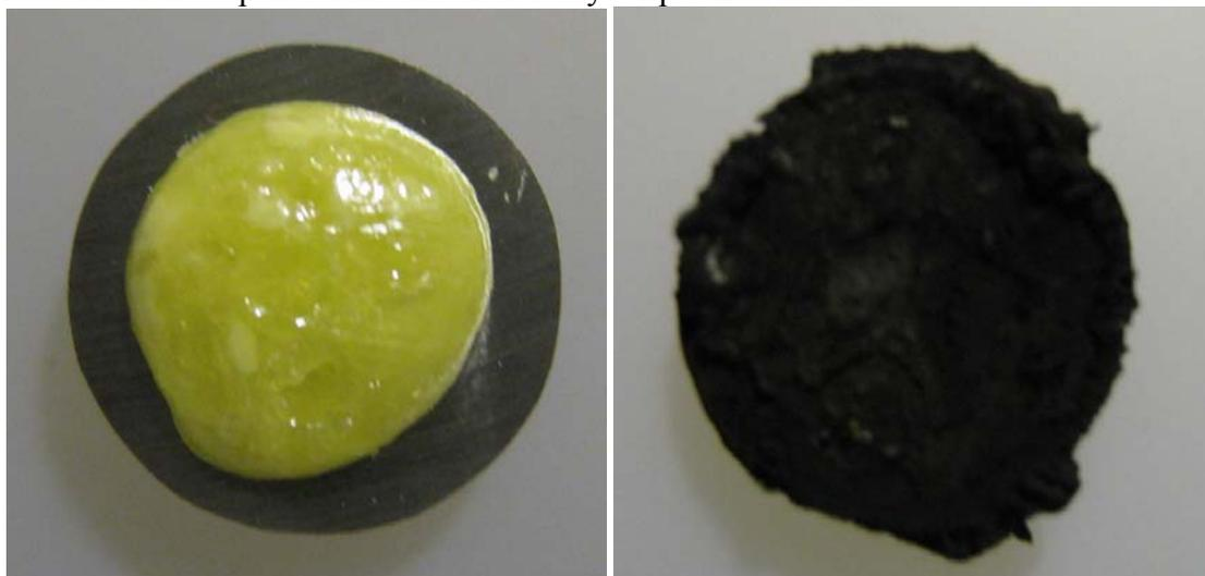
Figure 12. Corrosion coupon before and after 5 days exposure at 80°C.
