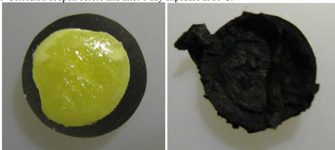
Figure 11. Corrosion coupon before and after 4 days exposure at 80°C.
