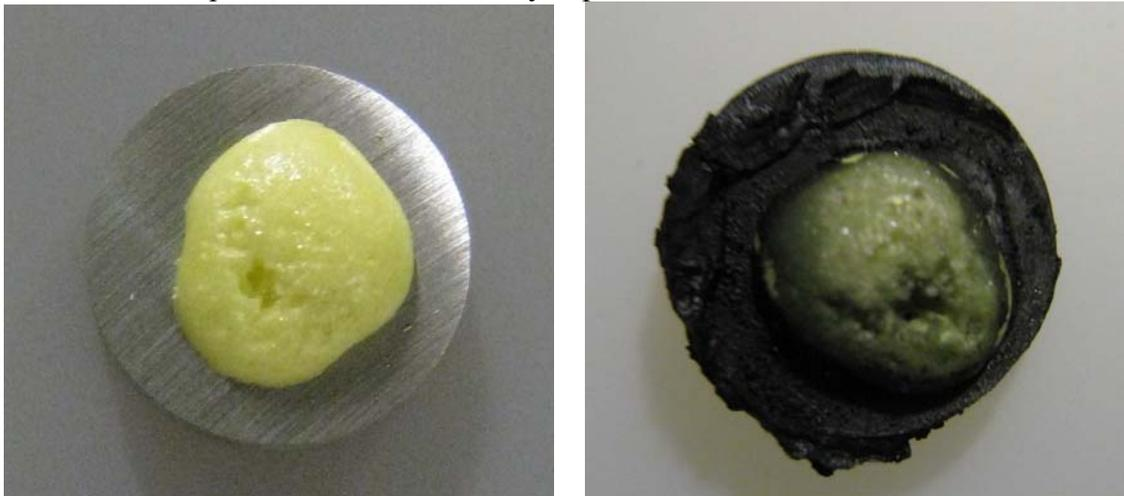
Figure 2. Corrosion coupon before and after 4 days exposure at 25°C.
