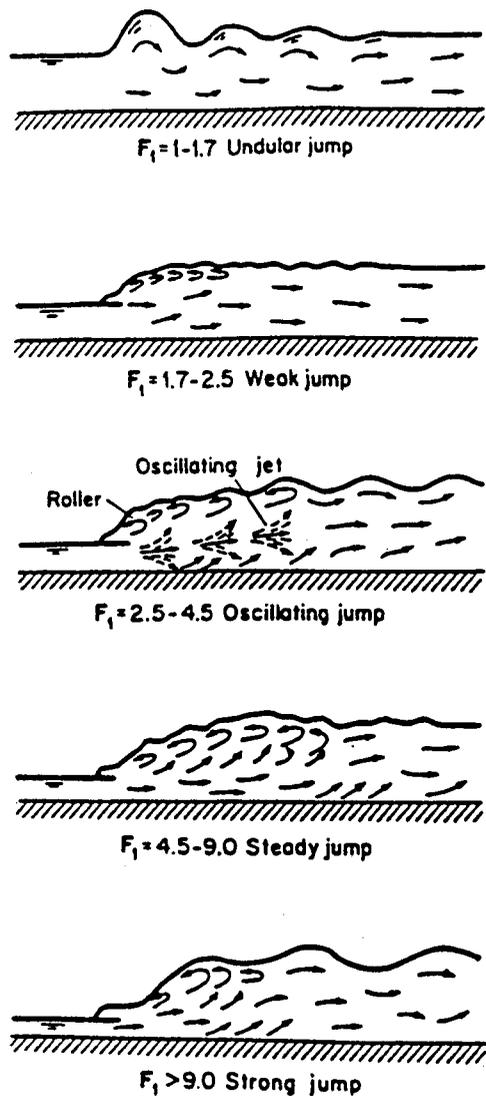
Fig. 1 Types of hydraulic jumps
