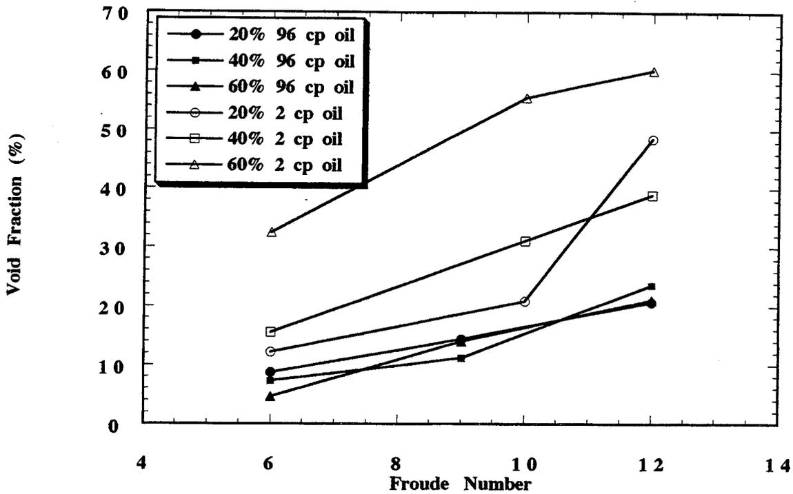
Figure 11a: Void fraction vs Froude number
