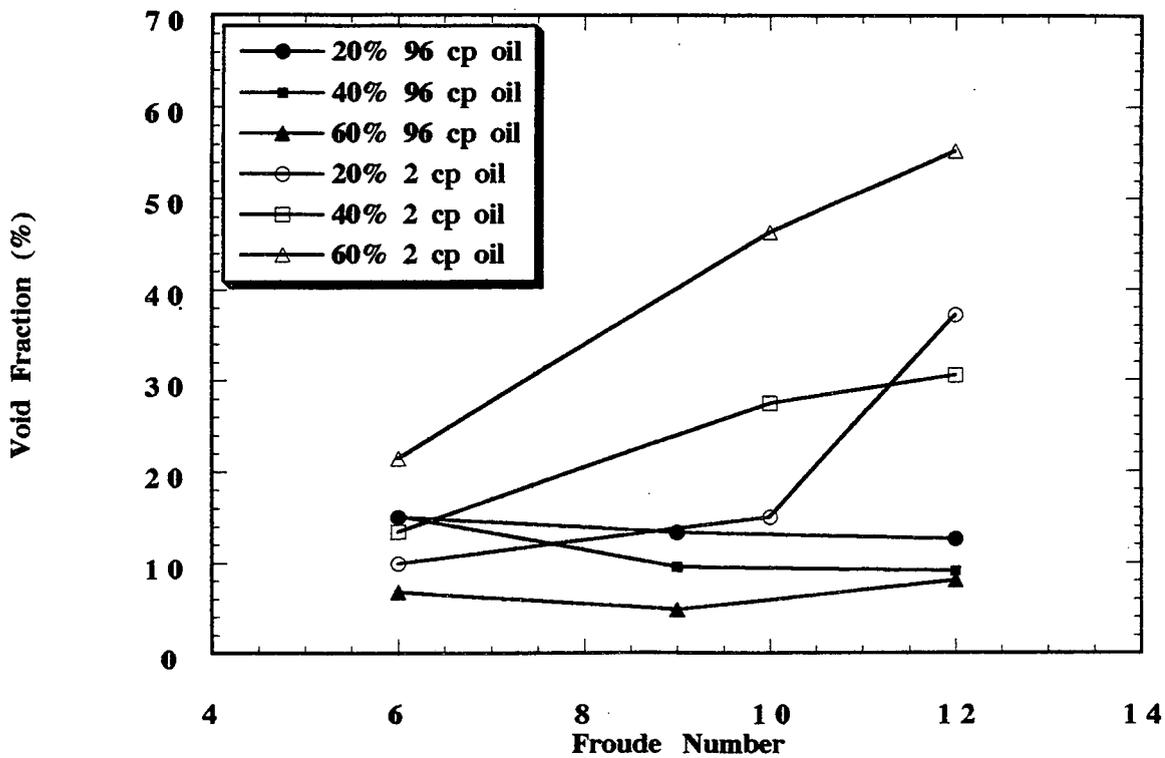
Figure 11b: Void fraction vs Froude number
