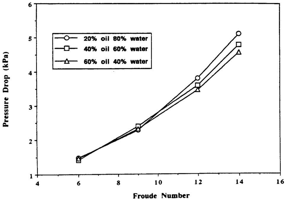
Figure 8a: Pressure drop vs Froude number
