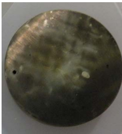
Figure 9. Steel sample surface after exposure in the sulfur/plastic-mesh/steel test where it was in close proximity to sulfur but electrically insulated from it.
