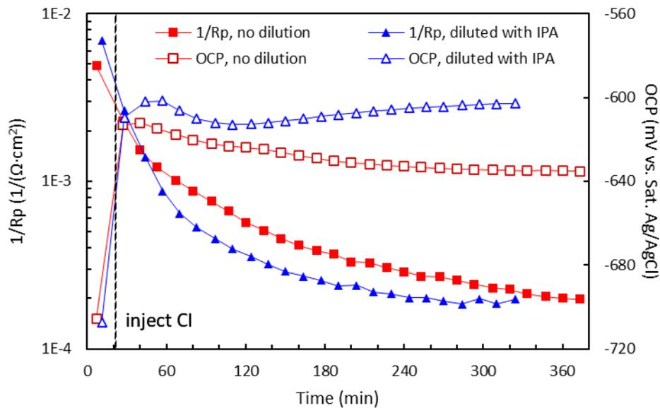
**Figure 5: Polarization resistance and open circuit potential evolution of C1018 inhibited with 30 ppm CCl in 50 g/L NaCl electrolyte saturated with CO<sub>2</sub> at 30°C. IPA is short for isopropanol.**
