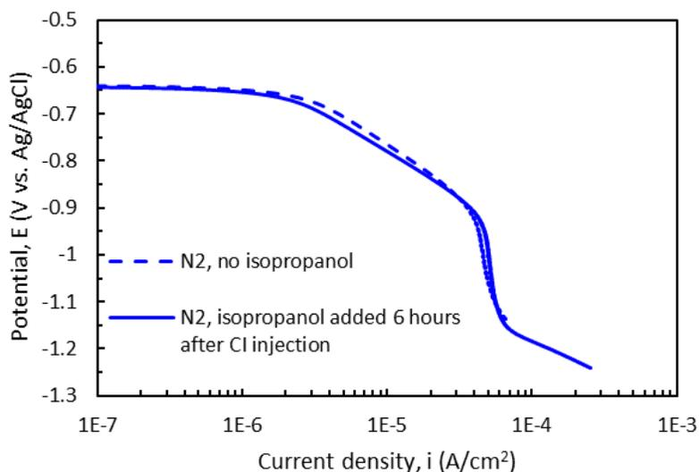
**Figure 7: Cathodic polarization curves of C1018 inhibited by 30ppm CCl in 50 g/L NaCl electrolyte deoxygenated with N<sub>2</sub> at 30°C. The polarization curves were collected sequentially in the same experiment as described in Figure 2b. Dashed line was collected first after addition of 30 ppm CCl, and solid line was collected after 3 mL uninhibited isopropanol was added.**
