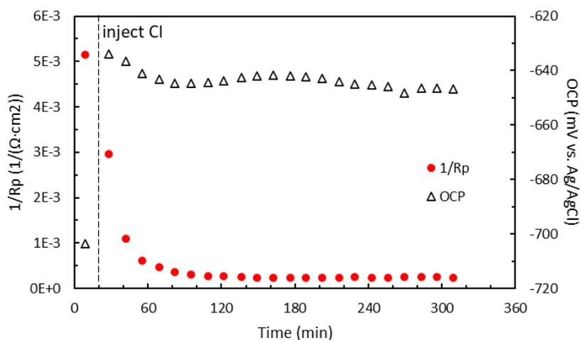
**Figure 3: Polarization resistance and open circuit potential evolution of C1018 inhibited with 10 ppm IMID-C14 above surface saturation concentration in 50 g/L NaCl electrolyte saturated with CO<sub>2</sub> at 25 °C.**
