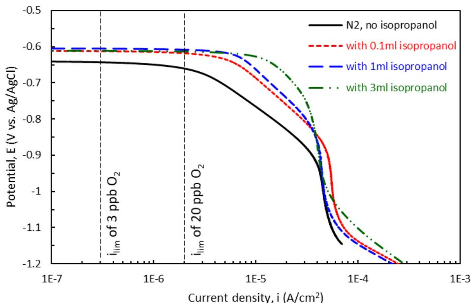
**Figure 8: Cathodic polarization curves of C1018 inhibited with 30 ppm CCl in 50 g/L NaCl electrolyte deoxygenated with N<sub>2</sub> at 30 °C. The CCl were diluted with different volume of isopropanol as indicated in the graph.**
