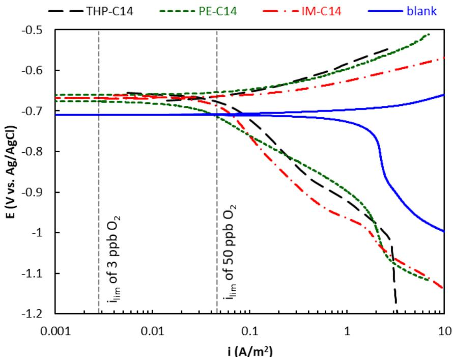
**Figure 4: Polarization curves of uninhibited C1018 (blank with no inhibitor), and C1018 inhibited by THP-C14 (8 mg solid dissolved in 3 mL isopropanol), PE-C14 (100 mg solid dissolved in 3 mL isopropanol), and IMID-C14 (20 mg solid dissolved in 3 mL isopropanol) in 2 L 50 g/L electrolyte saturated with CO<sub>2</sub> at 25 °C. Vertical lines are the limiting current of oxygen reduction reaction.**
