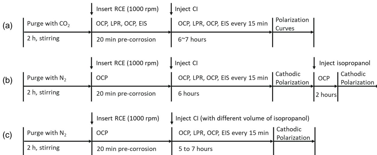
**Figure 2: Experimental procedures. (a) General inhibition experiment in CO<sub>2</sub> environment. (b) Inhibition experiment to evaluate the effect of the injection of isopropanol at the end of experiment when corrosion rate stabilized in N<sub>2</sub> environment. (c) Inhibition experiment to evaluate effect of different volumes of isopropanol in N<sub>2</sub> environment.**
