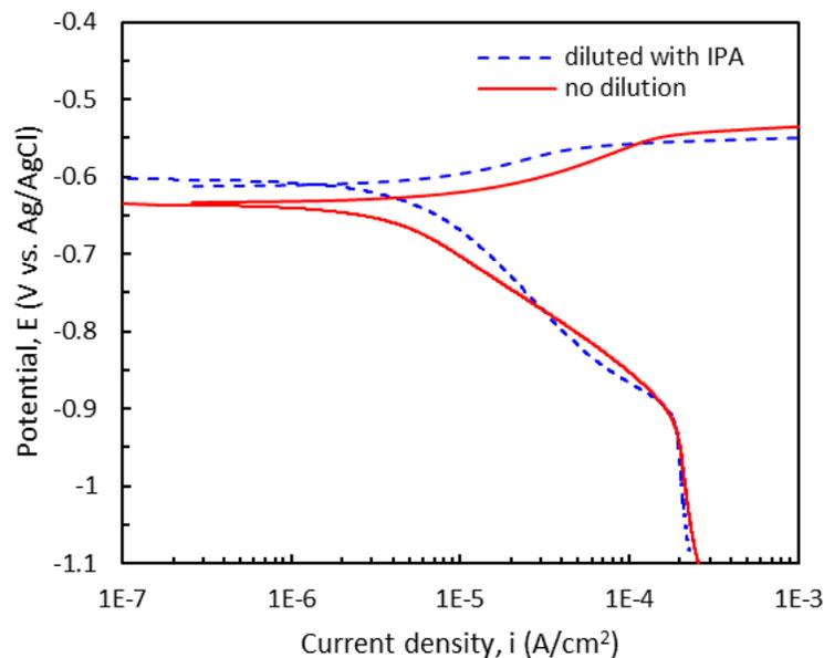
**Figure 6: Potentiodynamic sweeps of C1018 inhibited with 30 ppm CCl in 50 g/L NaCl electrolyte saturated with CO<sub>2</sub> at 30 °C, collected after the inhibition test shown in Figure 5. IPA is short for isopropanol.**
